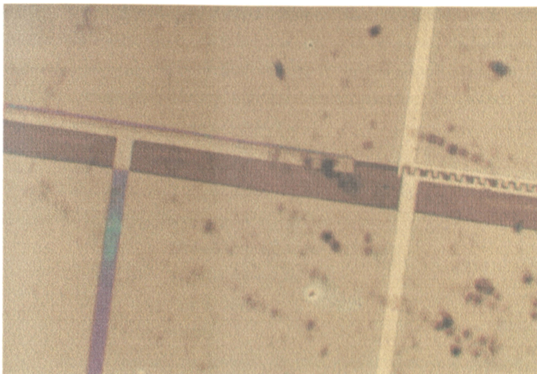
Figure 2. 5. Photograph of on-channel silver electrode and platinum interdigitated array electrode.
