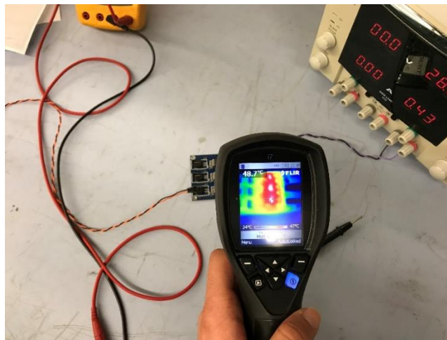
Figure: Picture of the FLIR Infrared Camera screen showing the temperature measurement of the three LDOs on one of the power boards
