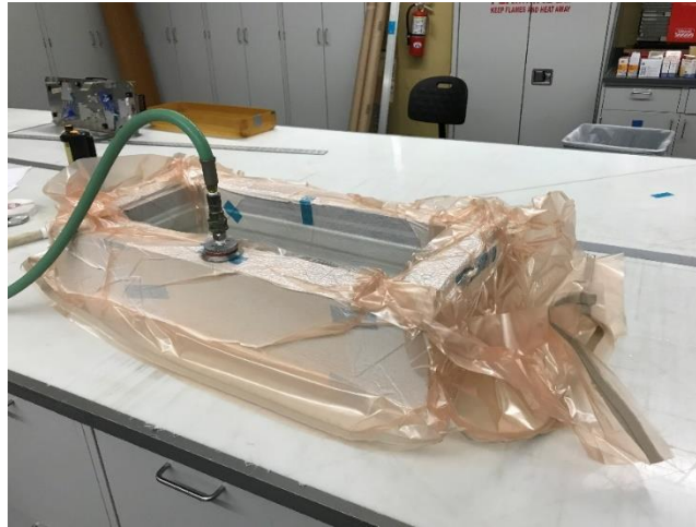
Figure: Picture of the vacuum bagging process of the fiberglass fairing. A prototype fairing and metal sheet with antenna arrays can be seen at the back.
