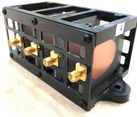
Figure 4-14: A picture of the fabricated four element array within the Delrin fixture
