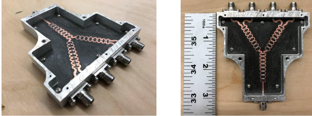
Figure 4-23: Pictures of the fabricated 1:4 power divider
