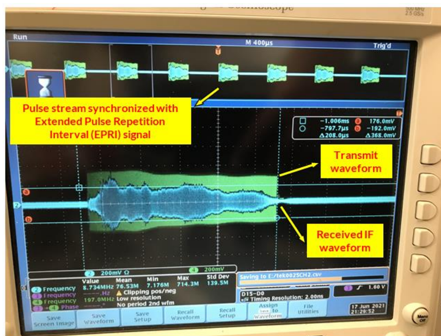
Figure 3-49: Picture of the transmit (PLL reference) and received IF waveforms on the oscilloscope
