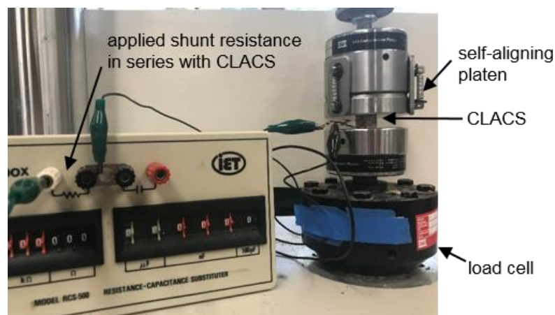
Figure 18. Experimental setup. Compressive load applied to CLACS and voltage measured across shunt resistance in series with CLACS.
