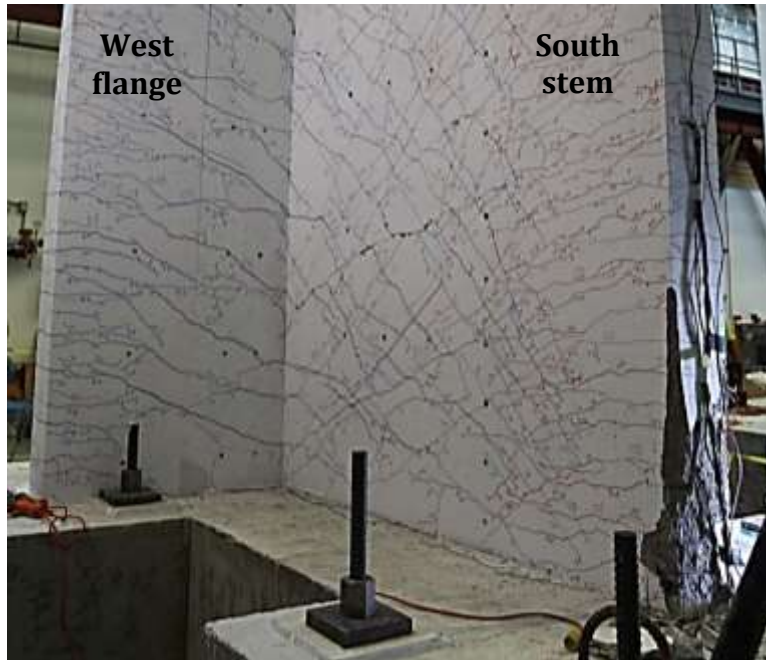
Figure 36 – Wall T5 without buckled bars in confined and unconfined stem during second cycle to 2% drift ratio (stem in compression)
