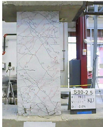
Figure C.97 – P80-2.5 at -2% chord rotation, second cycle
