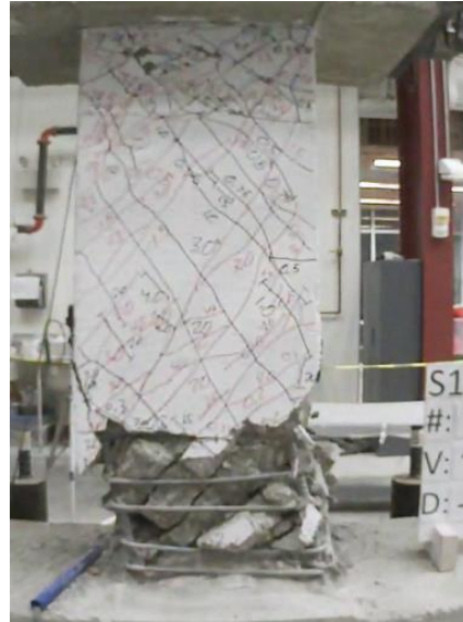
Figure C.109 – P100-2.5 at -6% chord rotation, second cycle
