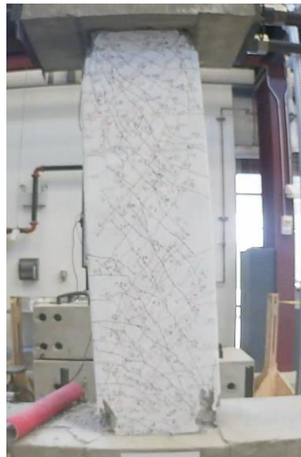
Figure C.65 – D80-3.5 at -4% chord rotation, second cycle
