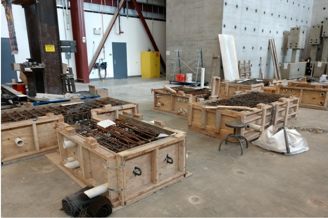
Figure B.7 – Specimens before casting, D80-1.5, D100-1.5, and D120-1.5 (from left to right)
