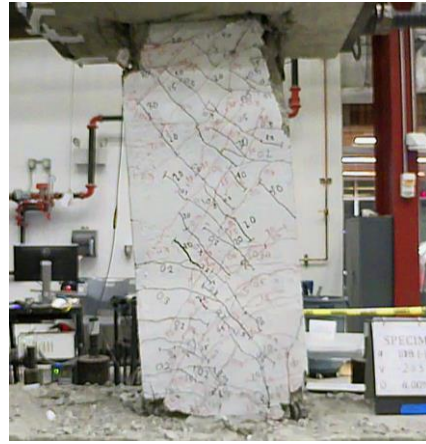
Figure C.35 – D80-2.5 at -6% chord rotation, second cycle
