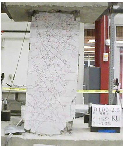
Figure C.44 – D100-2.5 at +4% chord rotation, second cycle
