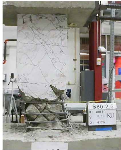
Figure C.101 – P80-2.5 at -6% chord rotation, second cycle
