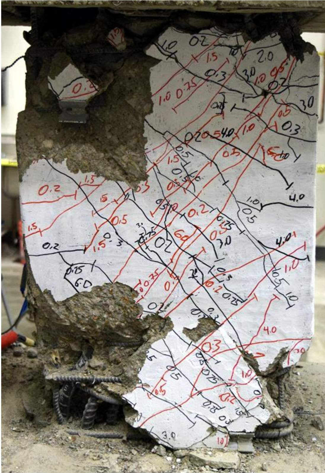
Figure C.2 – D80-1.5 during second cycle to 6% chord rotation
