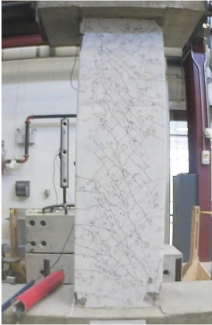
Figure C.62 – D80-3.5 at +2% chord rotation, second cycle
