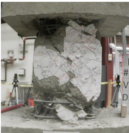
Figure C.9 – D80-1.5 at +8% chord rotation, first cycle
