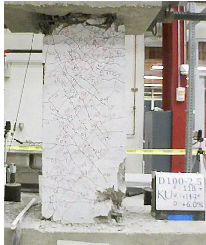
Figure C.47 – D100-2.5 at -6% chord rotation, second cycle
