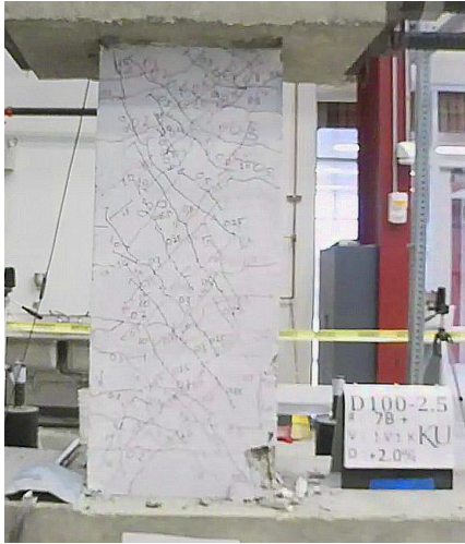
Figure C.42 – D100-2.5 at +2% chord rotation, second cycle
