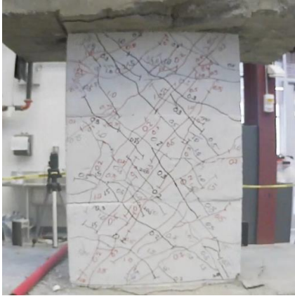
Figure C.13 – D100-1.5 at +2% chord rotation, second cycle
