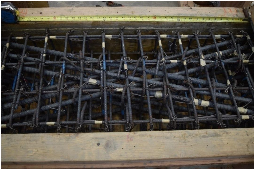
Figure B.2 – Coupling beam reinforcement, D120-2.5
