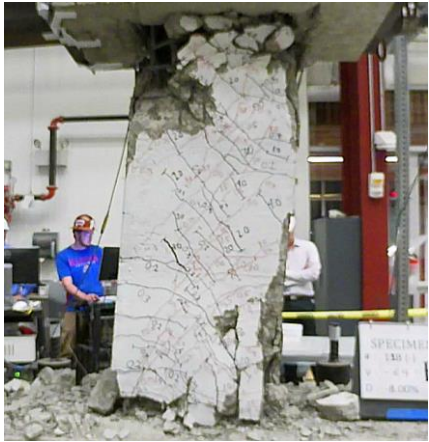
Figure C.38 – D80-2.5 at +10% chord rotation, first cycle
