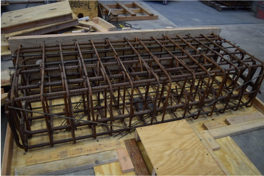
Figure B.5 – Base block reinforcement, typical of beams with aspect ratios of 2.5 and 3.5
