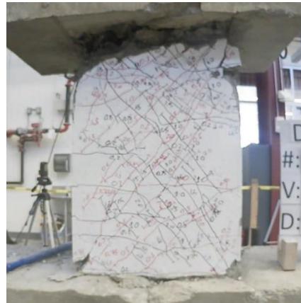
Figure C.25 – D120-1.5 at -4% chord rotation, second cycle
