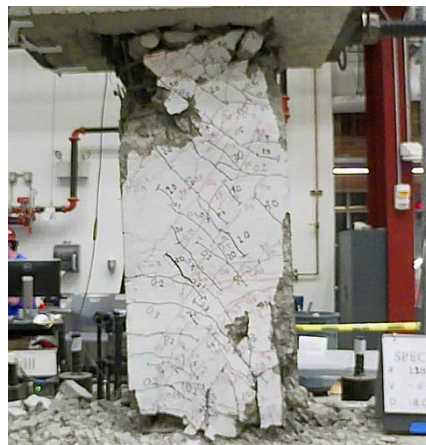
Figure C.37 – D80-2.5 at -8% chord rotation, second cycle
