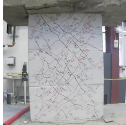
Figure C.14 – D100-1.5 at -2% chord rotation, second cycle
