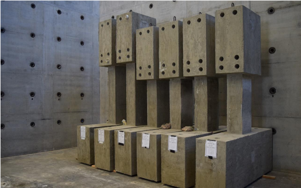
Figure B.8 – Specimens after formwork removal, D100-3.5, D80-3.5, P100-2.5, P80-2.5, D100-2.5, and D80-2.5 (from left to right)
