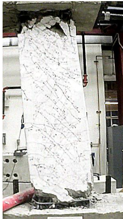
Figure C.81 – D100-3.5 at -8% chord rotation, second cycle
