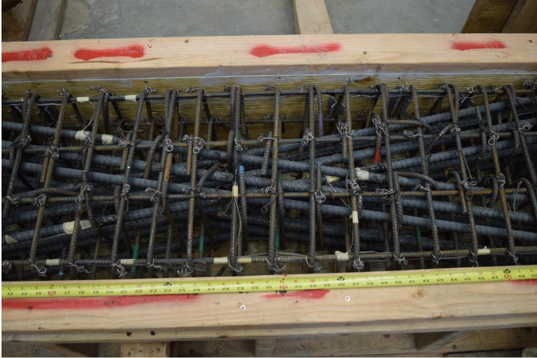
Figure B.3 – Coupling beam reinforcement, D120-3.5
