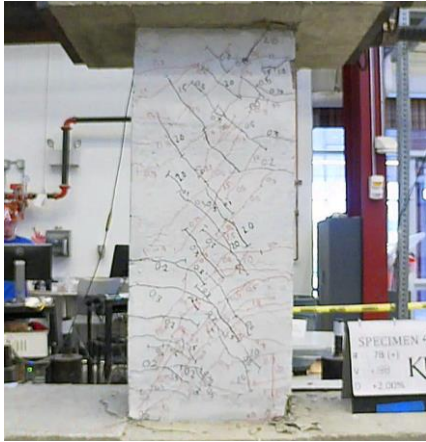
Figure C.30 – D80-2.5 at +2% chord rotation, second cycle
