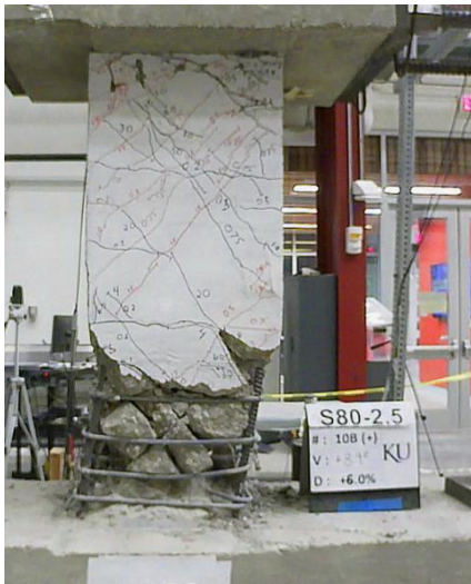
Figure C.100 – P80-2.5 at +6% chord rotation, second cycle
