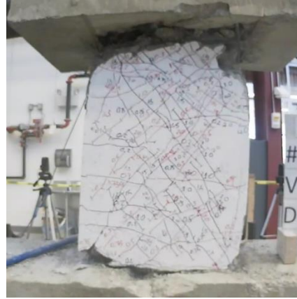
Figure C.27 – D120-1.5 at -6% chord rotation, first cycle
