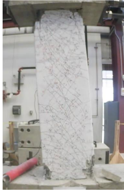
Figure C.67 – D80-3.5 at -6% chord rotation, second cycle
