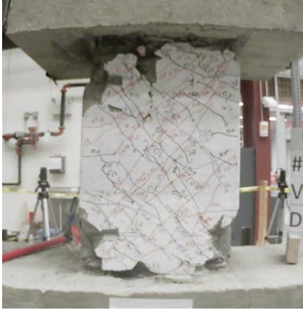
Figure C.7 – D80-1.5 at +6% chord rotation, second cycle
