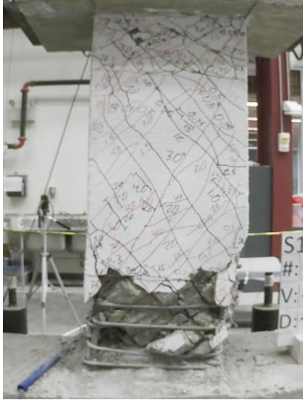
Figure C.108 – P100-2.5 at +6% chord rotation, second cycle
