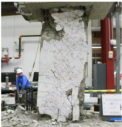
Figure C.36 – D80-2.5 at +8% chord rotation, second cycle
