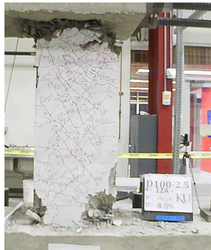
Figure C.49 – D100-2.5 at -8% chord rotation, first cycle
