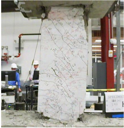
Figure C.34 – D80-2.5 at +6% chord rotation, second cycle
