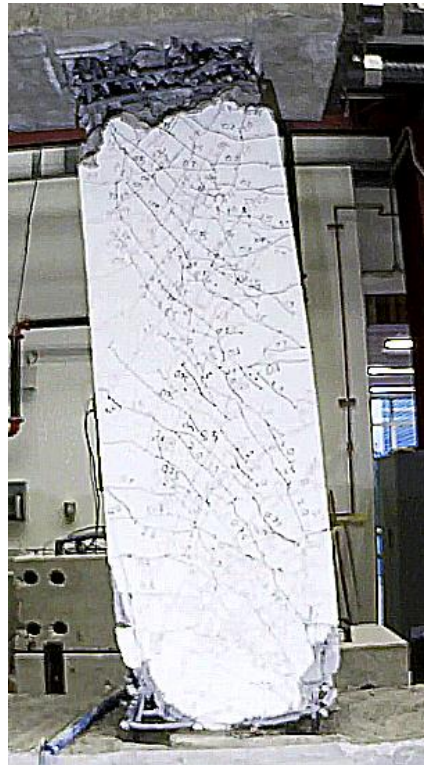
Figure C.93 – D120-3.5 at -8% chord rotation, second cycle
