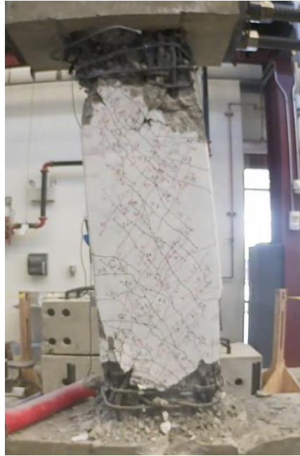
Figure C.71 – D80-3.5 at -10% chord rotation, first cycle
