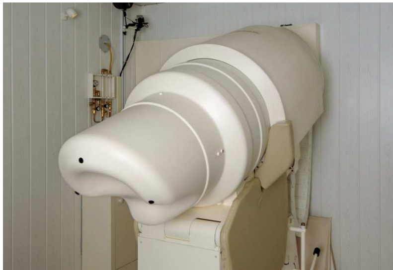
Figure 2. 83 Channel Investigational Biomagnetometer
