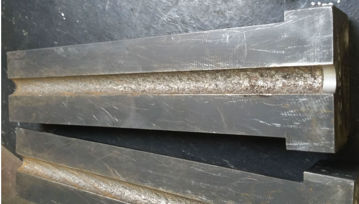
Figure 15 – Photograph of cylindrical grips with gritty tungsten-carbide coating welded to surface
