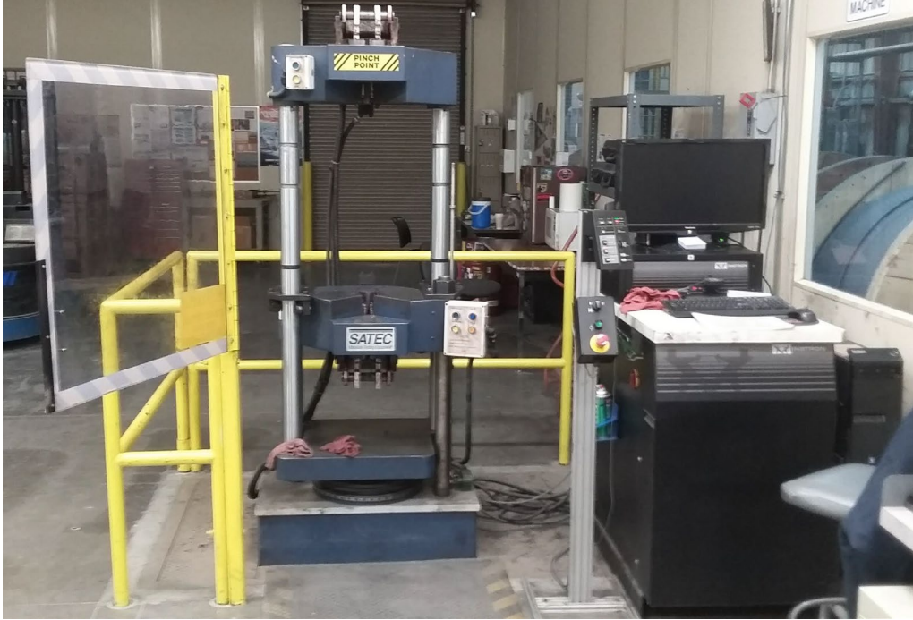
Figure 1 – Example of test frame and data acquisition system used for tensile testing of strands
