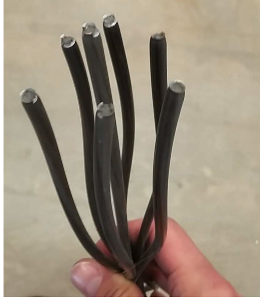
Figure 17 – Photograph of strand that exhibited nominally simultaneous fracture of seven wires
