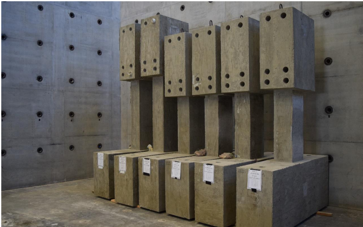
Figure B.6 – Specimens after formwork removal, D100-3.5, D80-3.5, P100-2.5, P80-2.5, D100-2.5, and D80-2.5 (from left to right)
