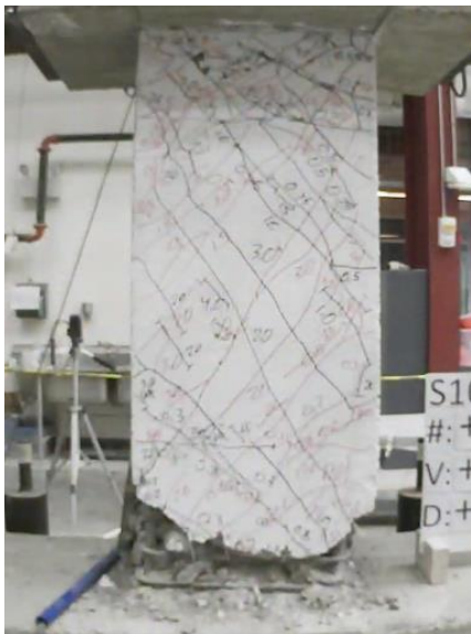
Figure C.84 – P100-2.5 at +4% chord rotation, second cycle
