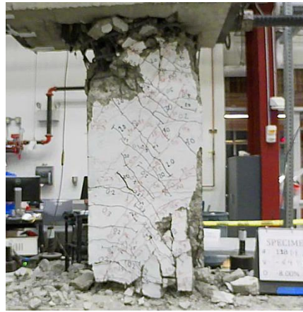
Figure C.31 – D80-2.5 at -10% chord rotation, first cycle
