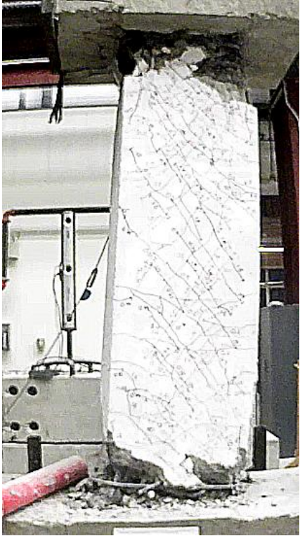
Figure C.66 – D100-3.5 at +10% chord rotation, first cycle
