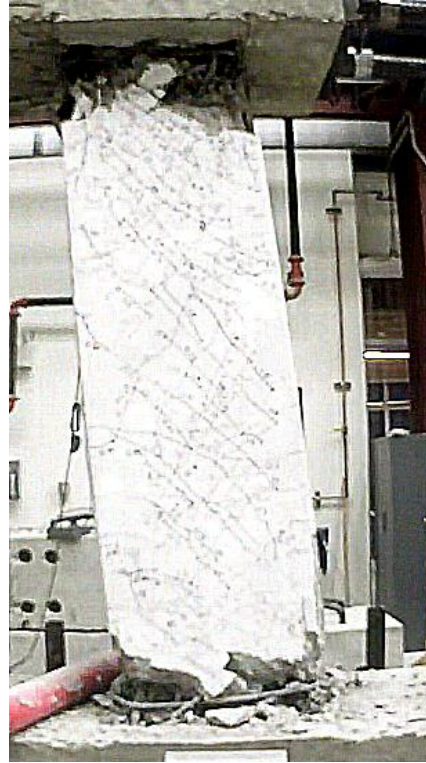
Figure C.67 – D100-3.5 at -10% chord rotation, first cycle
