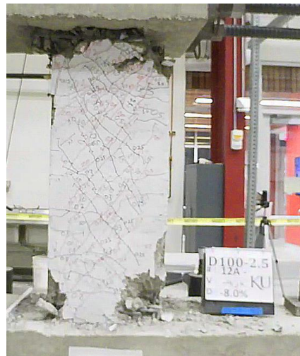
Figure C.39 – D100-2.5 at -8% chord rotation, first cycle
