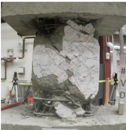
Figure C.7 – D80-1.5 at +8% chord rotation, first cycle
