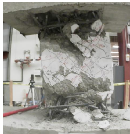
Figure C.8 – D80-1.5 at -8% chord rotation, first cycle
