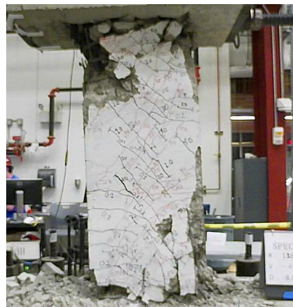
Figure C.29 – D80-2.5 at -8% chord rotation, second cycle
