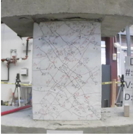
Figure C.1 – D80-1.5 at +2% chord rotation, second cycle
