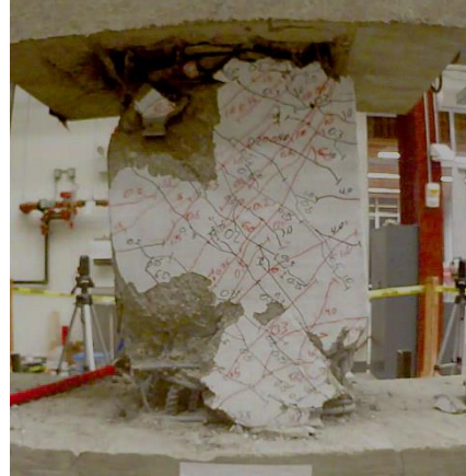
Figure C.6 – D80-1.5 at -6% chord rotation, second cycle
