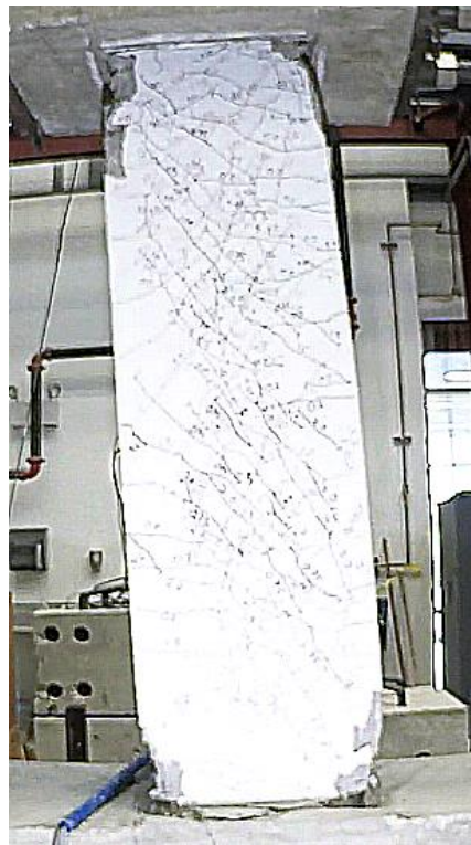
Figure C.71 – D120-3.5 at -4% chord rotation, second cycle
