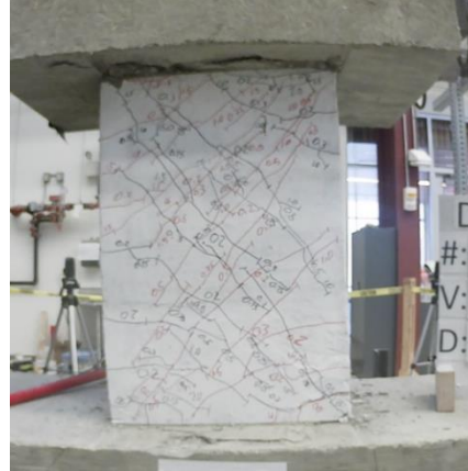
Figure C.2 – D80-1.5 at -2% chord rotation, second cycle
