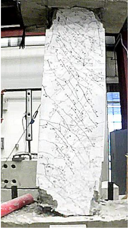
Figure C.62 – D100-3.5 at +6% chord rotation, second cycle
