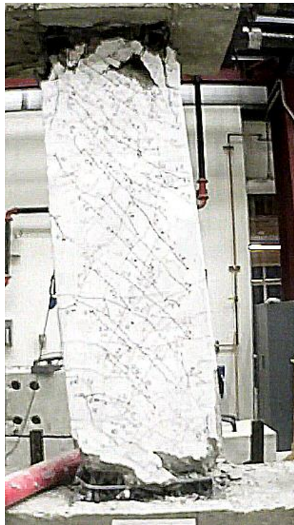
Figure C.65 – D100-3.5 at -8% chord rotation, second cycle
