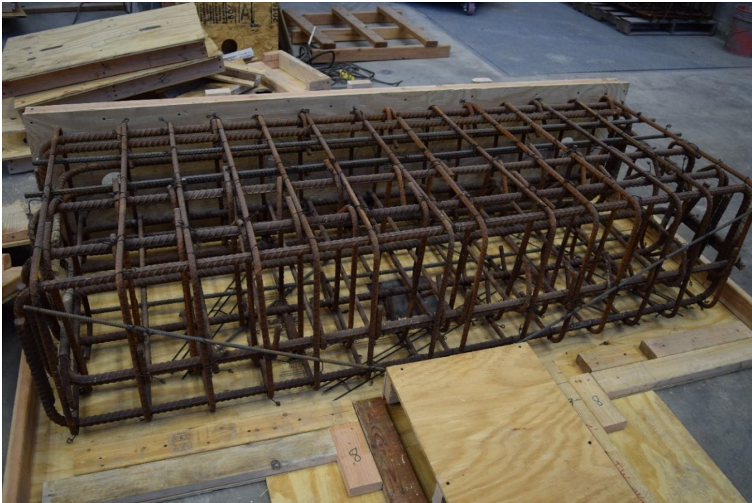
Figure B.4 – Base block reinforcement, P80-2.5
