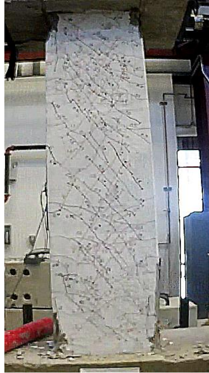
Figure C.59 – D100-3.5 at -2% chord rotation, second cycle
