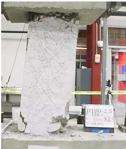
Figure C.38 – D100-2.5 at +8% chord rotation, first cycle
