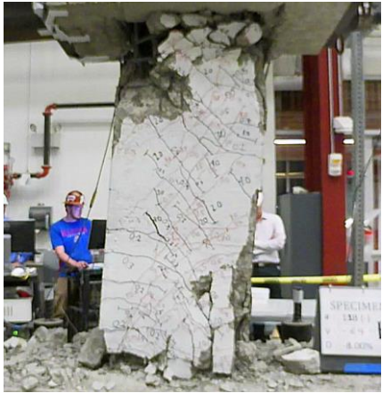
Figure C.30 – D80-2.5 at +10% chord rotation, first cycle
