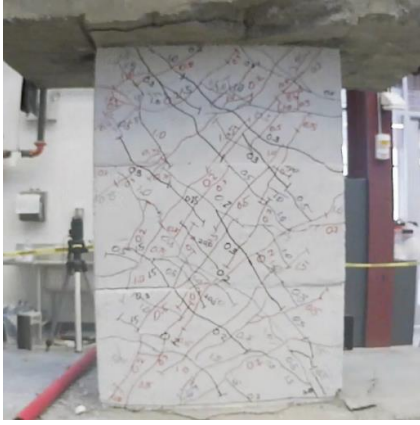
Figure C.9 – D100-1.5 at +2% chord rotation, second cycle
