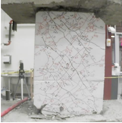
Figure C.13 – D100-1.5 at +6% chord rotation, second cycle
