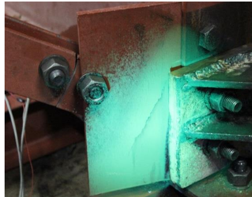
Figure 3-3: Cracks on 20-degree skewed cross-frame 775,000 cycles into Trial 2
