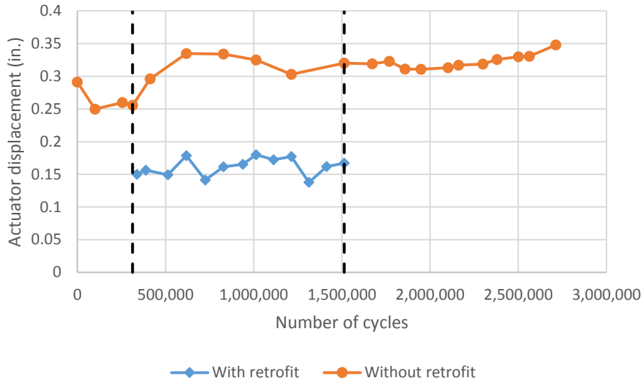
Figure 5-5: Actuator displacement vs. number of applied cycles at 2.5 kip of actuator force for the 40-degree skewed specimen
