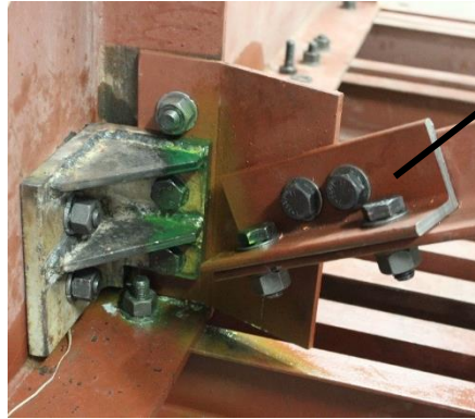
Figure 3-2: Crack on 20-degree skewed cross-frame 697,000 cycles into Trial 20-2 and the steel angle bolted to repair it
