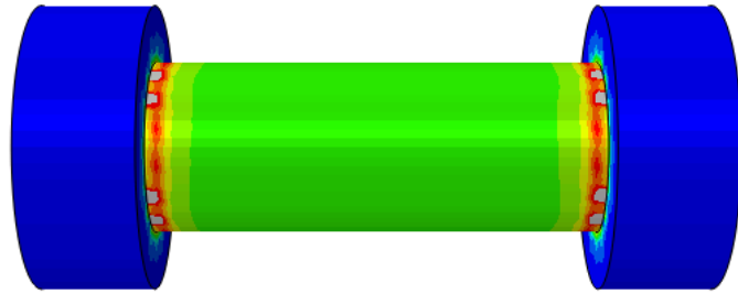
Figure 8-17: Maximum principal stresses of top bolt connecting angle and stringer web for model of double-angle connection with shorter floorbeam web
