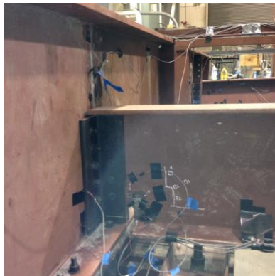
Figure 7-1: Photograph of the double-angle connection specimen
