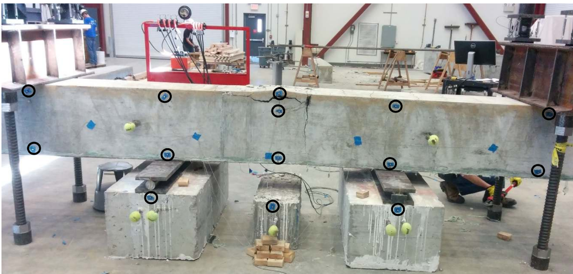
Figure 2.11 Location of infrared markers marked by circles
