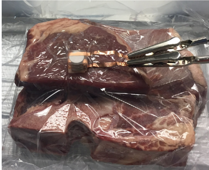
Figure 39 - Tissue media used in testing
