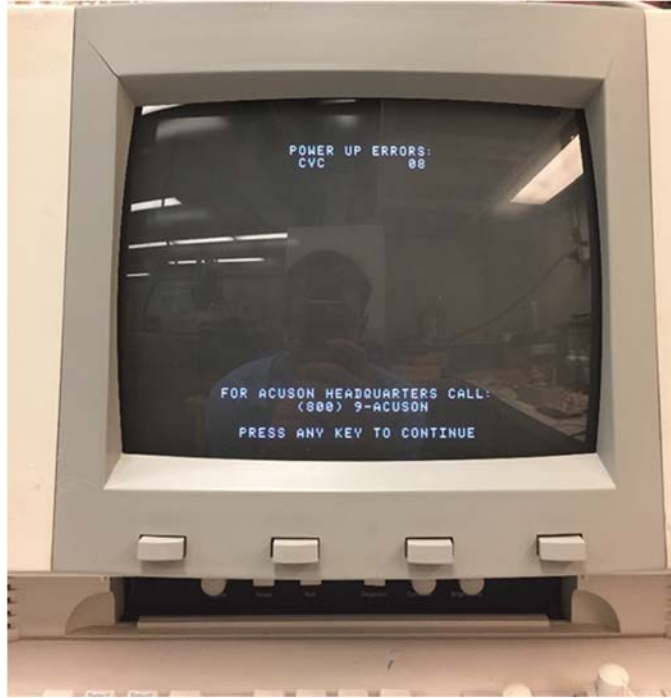
Figure 79 - Contents of Ultrasound Imaging Screen after waiting a few minutes for the machine to startup
