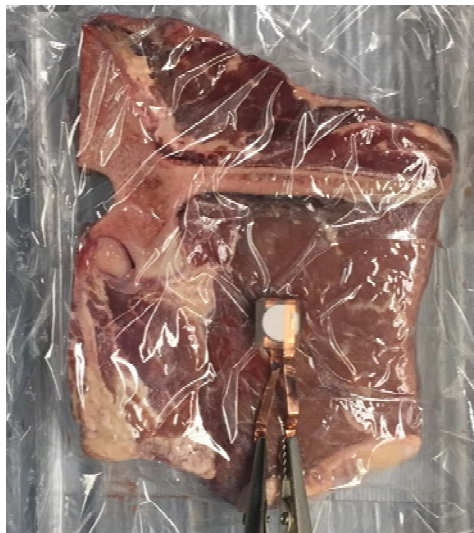
Figure 58 - CLACS placed on top of 20mm tissue thickness media for testing
