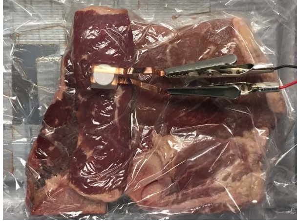
Figure 59 - Tissue plus bone media with a little slab of tissue placed above the small part of the "T" bone to achieve 20mm media thickness.
