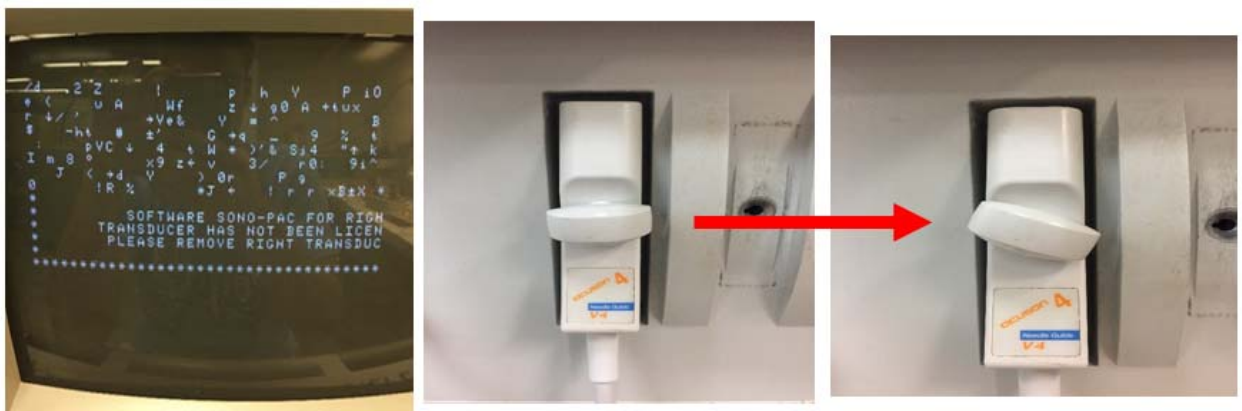
Figure 93 - Ultrasound imaging screen if the probe is not fully connected to the machine
