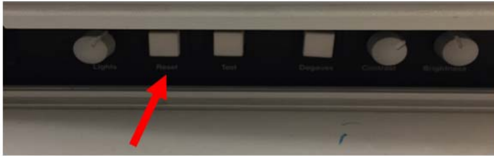
Figure 90 - Reset the ultrasound medical imaging machine after entering and saving the encryption strings
