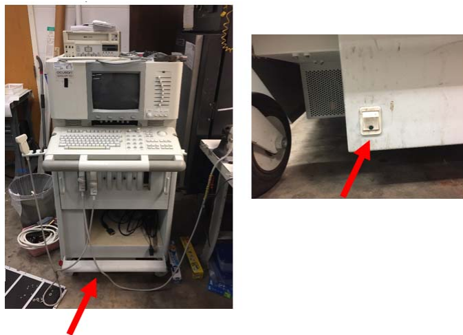
Figure 78 - Location of power switch on Acuson 128XP/10 ultrasound medical imaging machine
