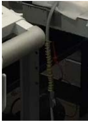
Figure 47 - Looped wire wrapped around the Ultrasound probe wire to capture the magnetic field generated by moving electrons in the probe wire
