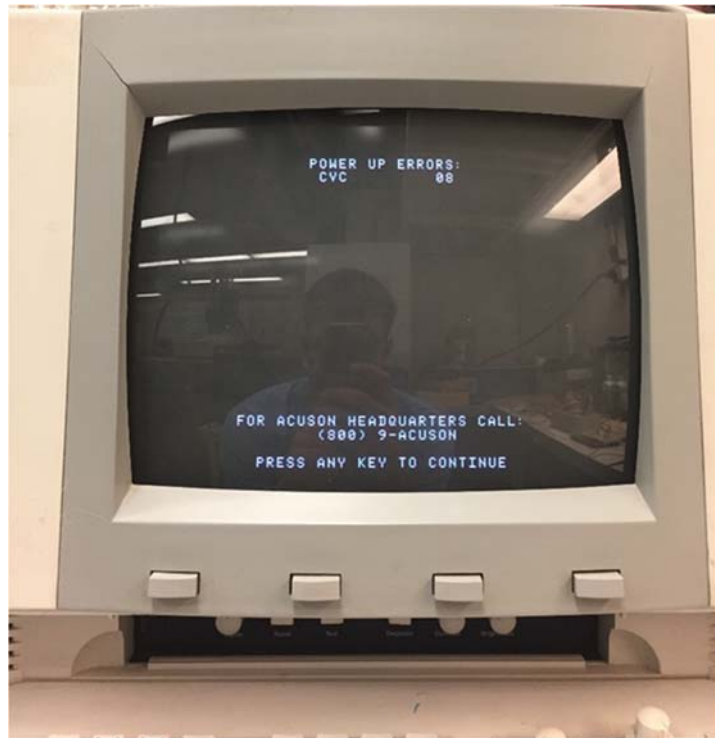
Figure 81 - Contents of Ultrasound Imaging Screen after waiting a few minutes again for the machine to startup
