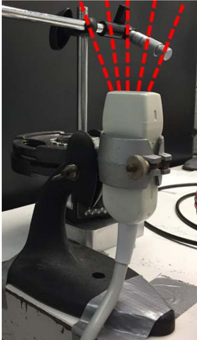
Figure 19 - Phased array probe (Adapted from 28 )
