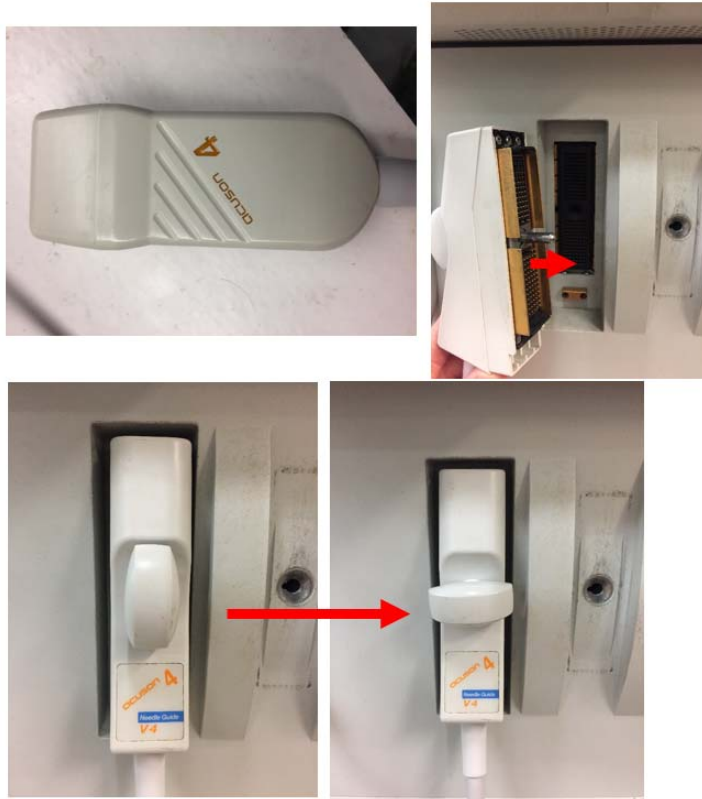
Figure 77 - Plugging in V4 Ultrasound Probe
