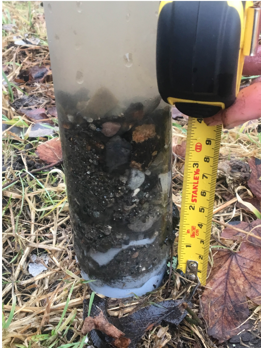
Figure L.2: The soil core taken at the Raadvad site at the same time SBPVP testing was conducted.
