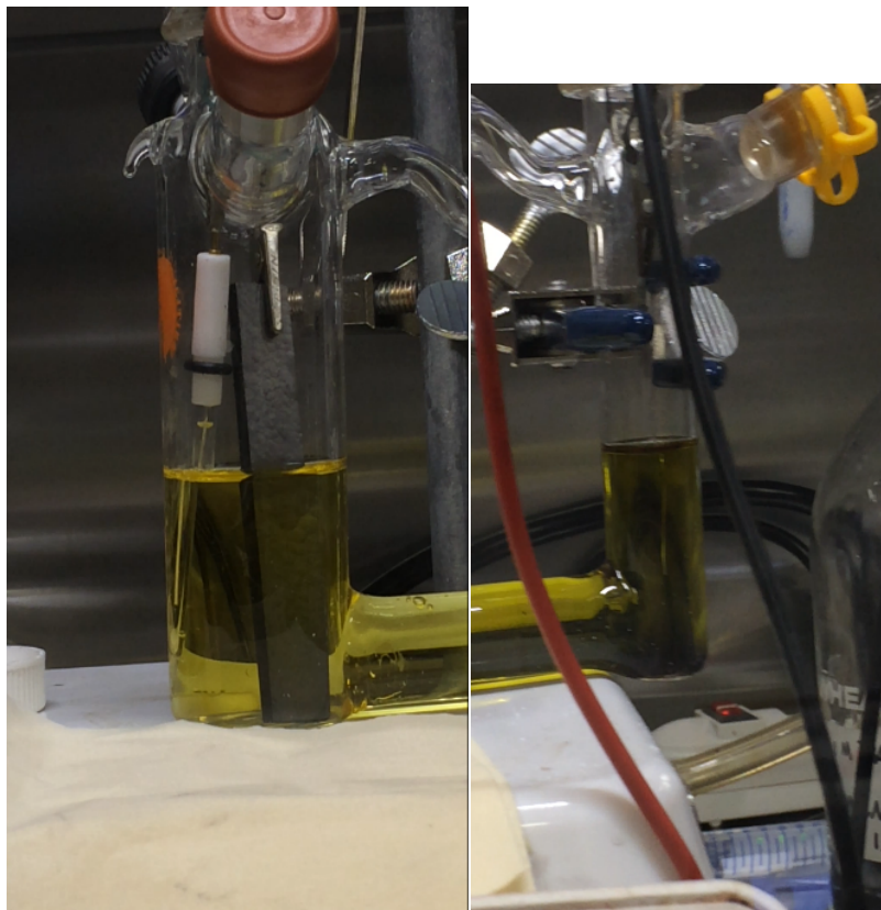
Figure 1.30: Carbon working electrode, silver reference electrode, catalyst, and anilinium triflate (left). Platinum counter electrode and ferrocene (right).
