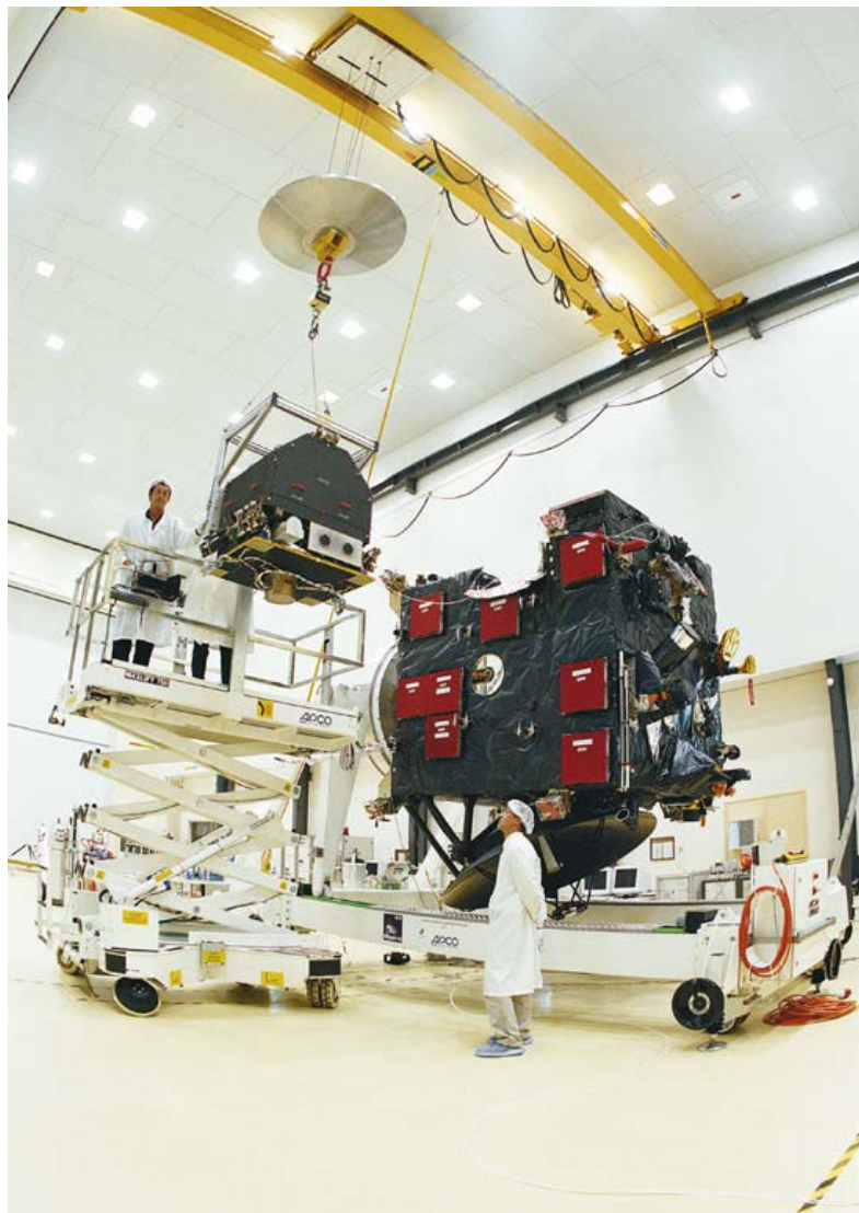
Figure 1.4 – Rosetta spacecraft and Philae lander as it is being mounted on the spacecraft. The high gain antenna is visible in this picture beneath the spacecraft. Adapted from (Glassmeier et al., 2007a).
