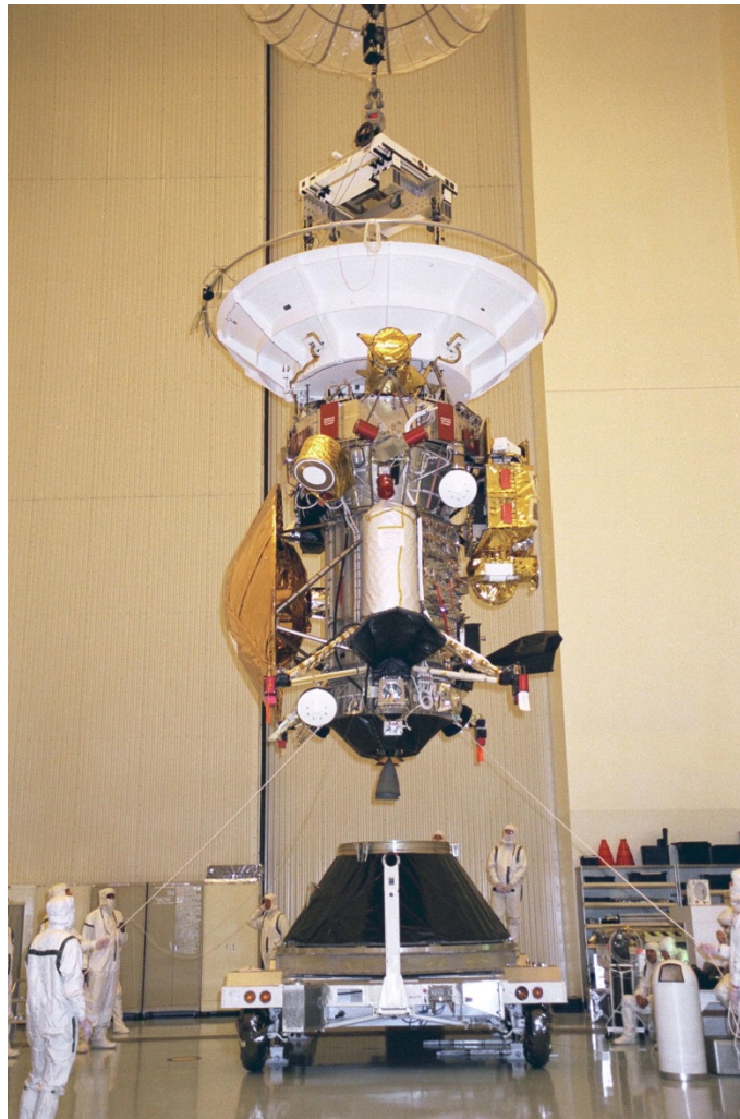
Figure 1.11 - An image of the installation of the Cassini spacecraft and Huygens probe on the payload adapter. The spacecraft weighed 5.7 tons and was launched on October 15, 1997. The white high gain antenna is visible at the top; the golden drum shape on the left side of the spacecraft is the Huygens probe. Photo courtesy: NASA.
