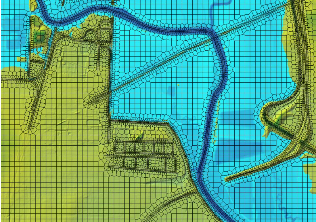
Figure 3-8: 1K cms flood at the Coffeyville Resources Refinery along the Verdigris River.
