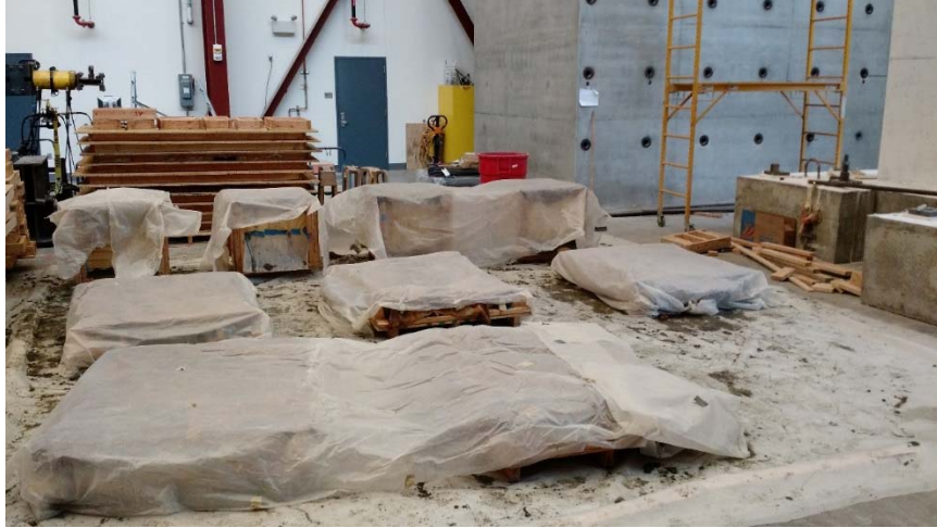
Figure 2.6: Wet curing of specimens
