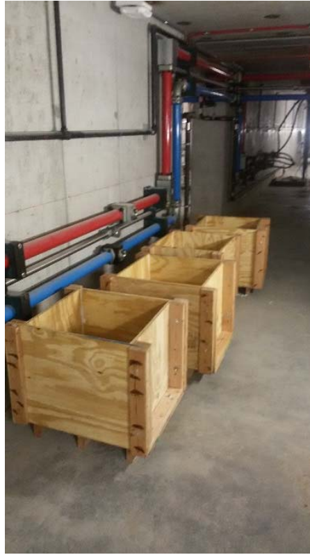
Figure 2.5: Block specimen formwork
