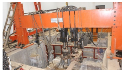
Figure 5. Testing set-up: (a) schematic of the loading system; (b) photograph of the plate load test
