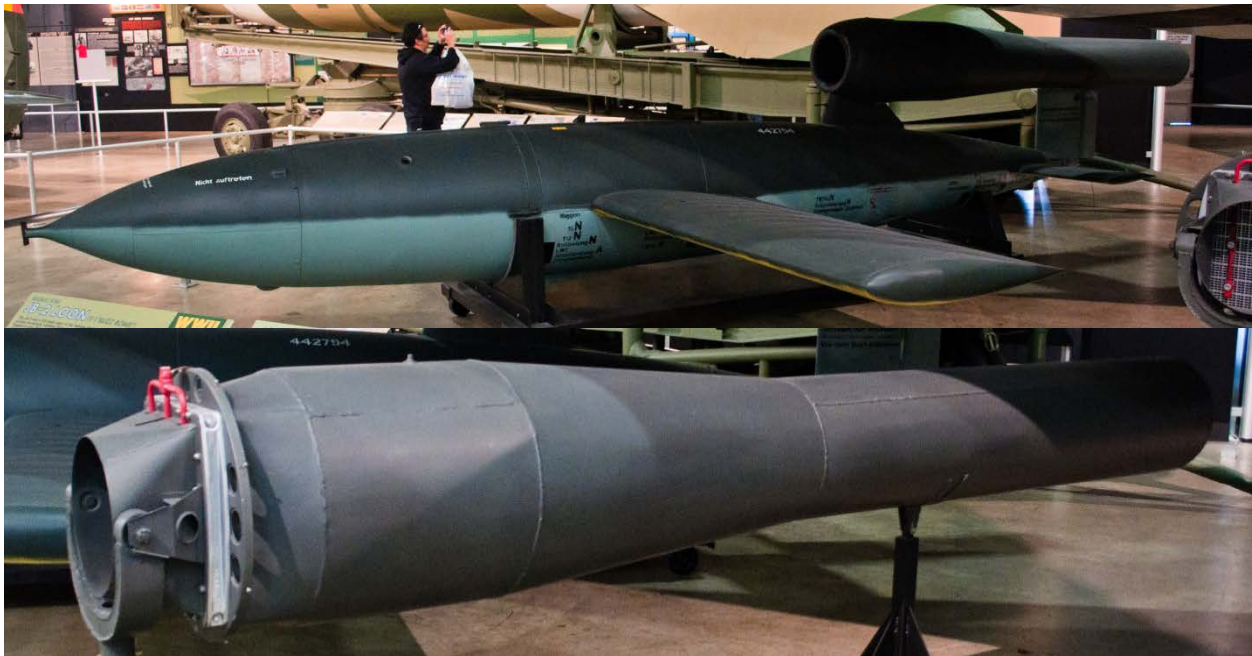
Figure 3: V-1 Cruise Missile (Top) and its Powerplant, the Argus As 014 Valved Pulse Jet Engine (Bottom), Images Taken by the Author at the National Museum of the US Air Force
