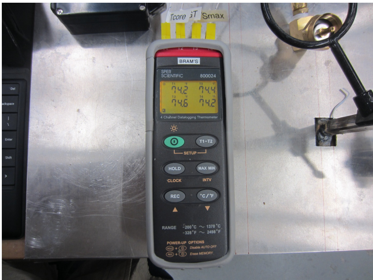
Figure 114: Sper Scientific 800024 4-Channel Datalogging Thermometer with Four Labeled Type-K Thermocouples Corresponding to Different Locations On and In The Pressure Jet Engine (Temperatures are in deg F and Shown Reading Room Temperature)
