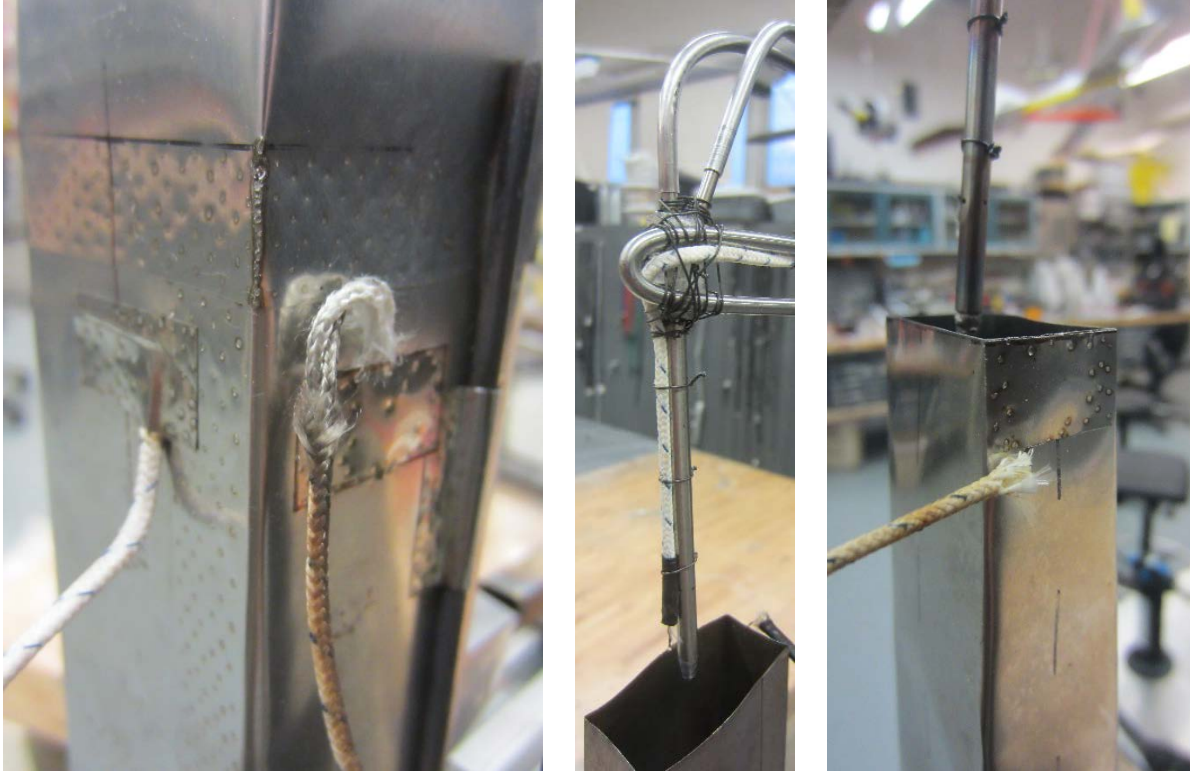
Figure 115: Thermocouple Installation Methods: Core Surface “Pocket” and Internal Core (Left), Nozzle Exit Surface “Pocket” (Middle), and Coincident to Pitot Probe (Right)
