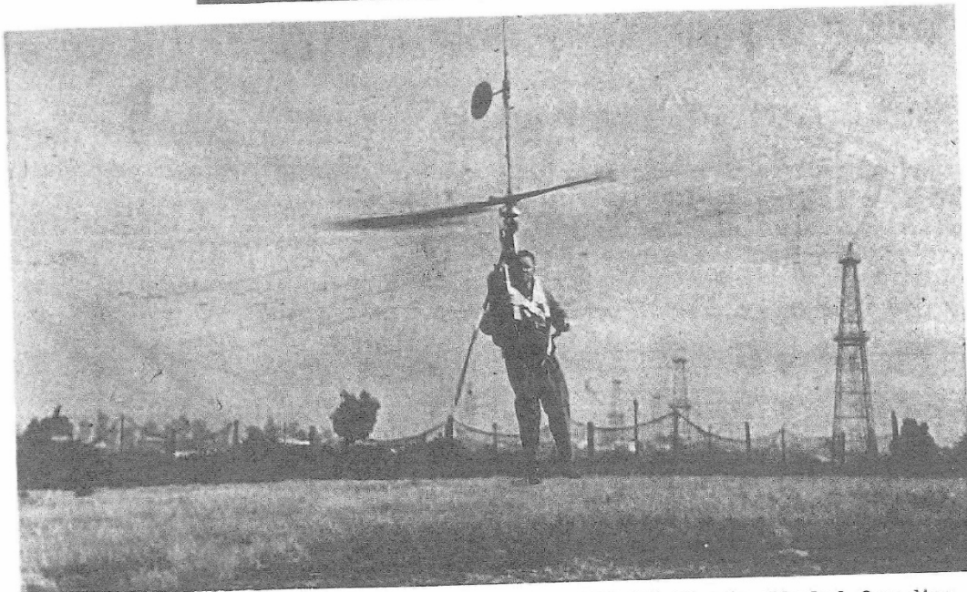
E.M. Gluhareff Harness Flight Testing MEG-1X Single Bladed One-Man Portable Helicopter, Powered by one G8-2-25 Jet Engine.
