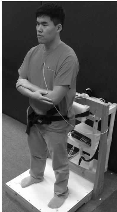
Figure 2. Experiment Set up and Sacral Restraint. The participants stood on a platform with their backside against a height-adjustable sacral support and were belted in with the accompanying restraint to limit sacral motion. The transmitter was positioned behind the platform.
