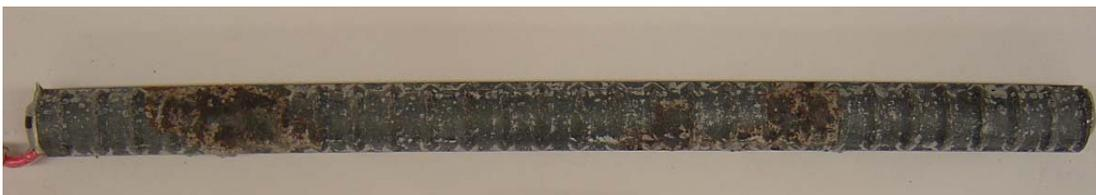
**Figure 3.129** – Initiation Beam Test. Conventional steel in the top mat (B-N4-Rheocrete-45N-4) showing severe corrosion.
