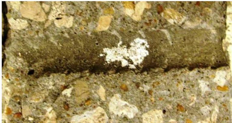
**Figure 3.140** – Initiation Beam Test. Specimen with zinc-coated reinforcement after autopsy (B-Zn-45N-10) showing visible interior staining of the concrete.
