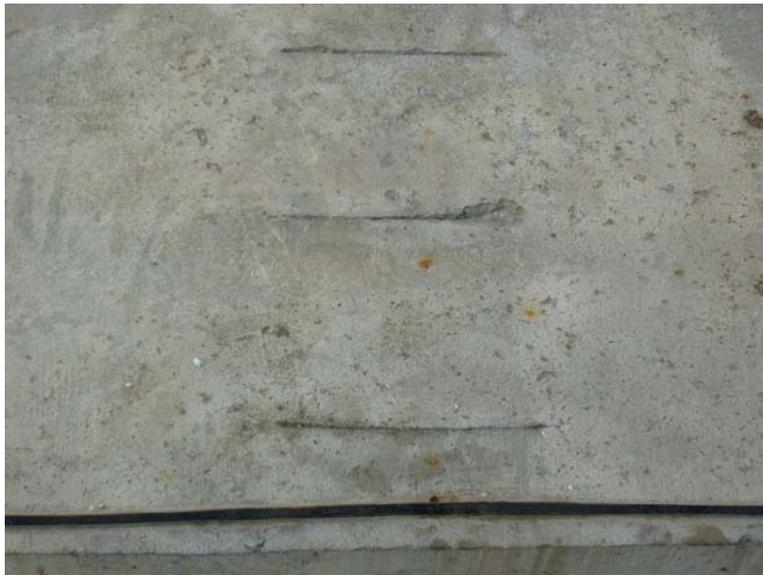
**Figure 3.91** – Field test specimen ECR(DCI) (1) with simulated cracks at week 179, showing light staining on the surface.
