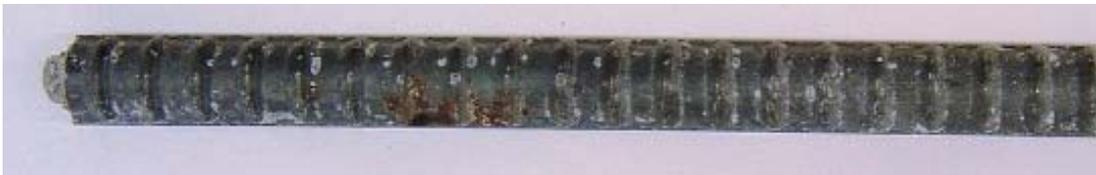
**Figure 3.139** – Typical corrosion at initiation on conventional steel.
