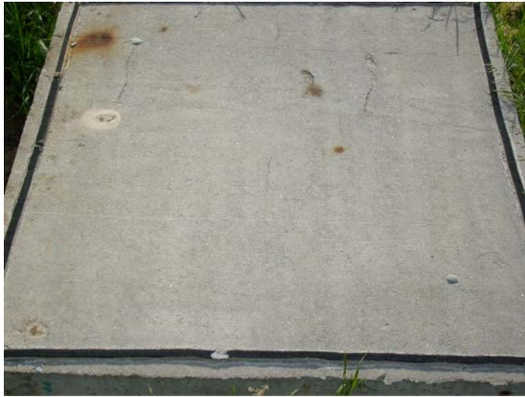
**Figure 3.90** – Field test specimen Conv. (1) at week 205, showing cracking, spalling, and heavy staining on portions of the surface.
