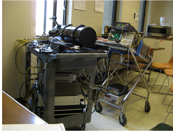
Figure 5.10 – Photo of the lidar aimed towards the target building.
