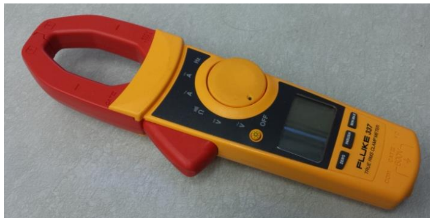
Figure 139: Fluke multimeter for measuring high current.
