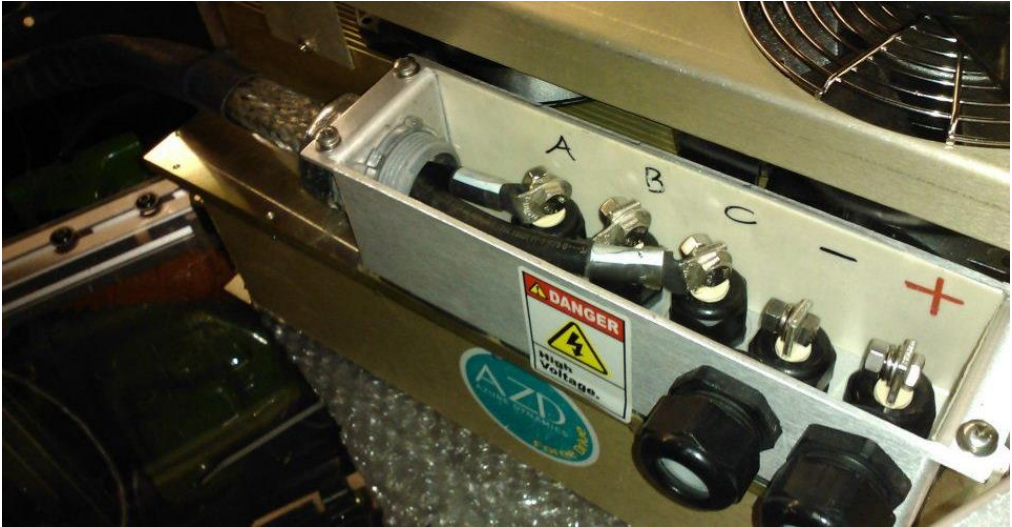
Figure 54: DMOc445 three-phase AC connections.
