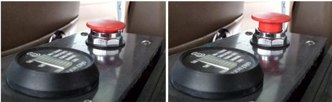
Figure 75: The contactor control button is in the 'OFF' position on the left, and in the 'ON' position on the right.
