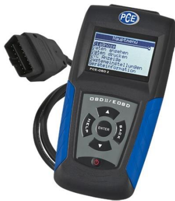
Figure 9: An example of an OBD-II scan tool with the standardized Data Link Connector [14].
