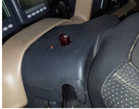
Figure 151: The hazard light switch is on top of the steering column.
