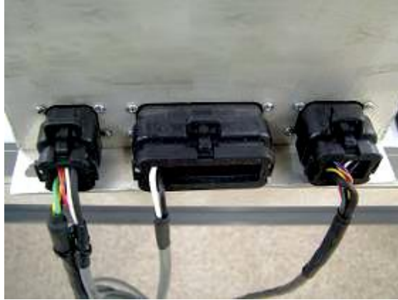
Figure 27: DMOC445 connection terminals. The 8-pin terminal for vehicle communication is on the left, the 35-pin interface terminal is in the middle, and the 14-pin terminal for motor data is on the right [24].
