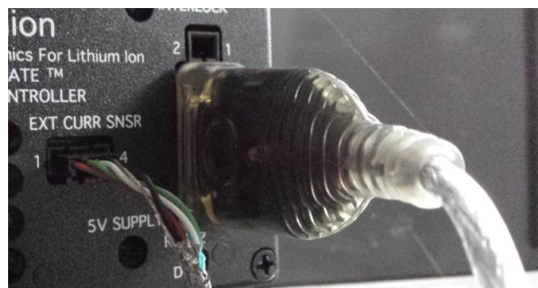
Figure 118: The ATEN RS-232 to USB connection on the BMS controller.
