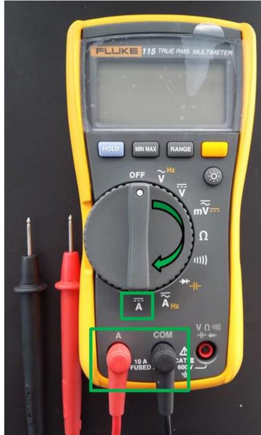
Figure 133: To measure current, ensure the probes are inserted into the current input terminal before rotating the dial to the indicated position.
