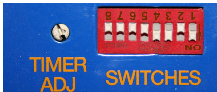
Figure 138: Magnified image of the timer adjustment and dip switches on the battery charger.
