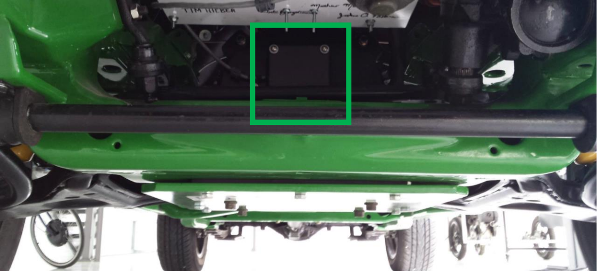
Figure 57: The AC55 encoder is located on the front of the motor.
