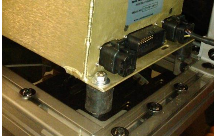
Figure 60: The DMOC has four vibration isolating mounts located at each corner of the controller.
