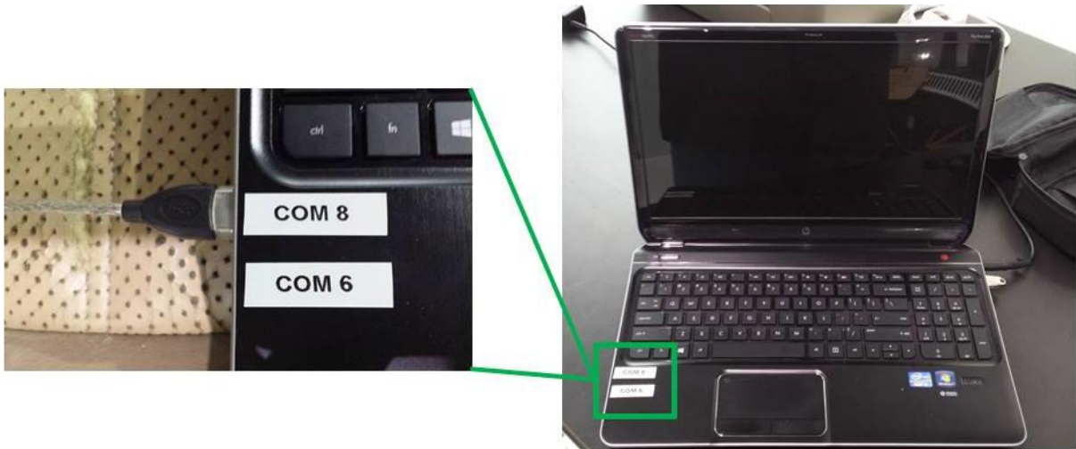
Figure 119: JimmE-V laptop with the BMS plugged into COM port 8.
