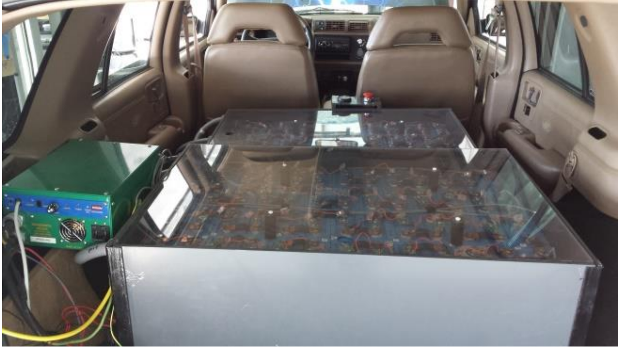
Figure 102: The JimmE-V battery packs in the rear passenger compartment (far) and rear cargo section (near).
