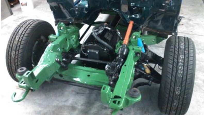
Figure 52: AC55 motor installation location between the frame rails.
