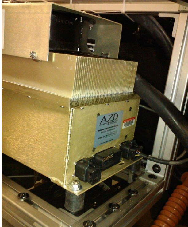
Figure 56: Motor encoder harness connected to the 14-pin connector on the DMOC445.
