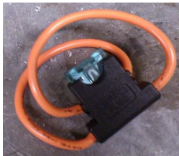
Figure 38: In-line fuse holder and 30 AMP fuse to prevent excessive current from the 12 VDC battery.
