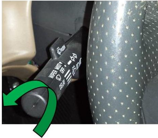
Figure 150: The wiper speed is controlled by rotating the end of the turn indicator switch.
