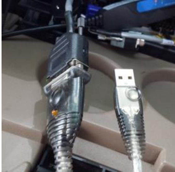
Figure 61: The ATEN USB to RS-232 adapter is located in the glove box of the JimmE-V.
