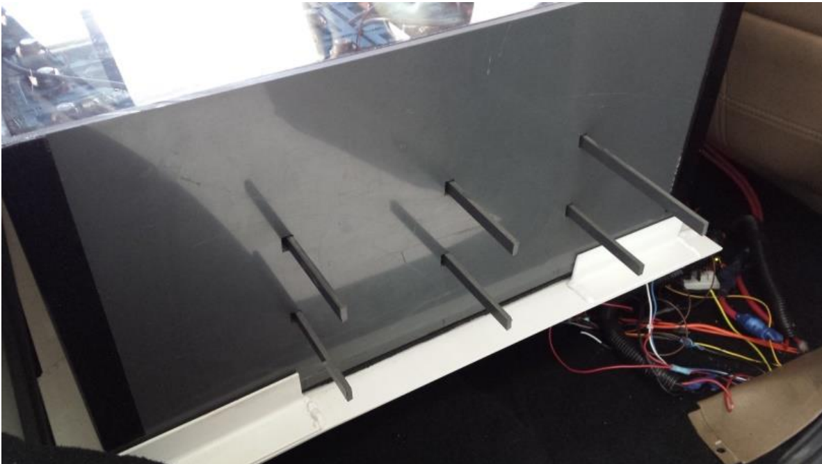
Figure 104: The locking bars can be accessed from the sides of the battery boxes. They safely secure the batteries to the boxes.
