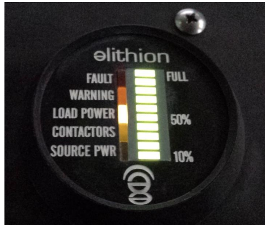
Figure 117: The SOC gauge displays the current SOC along with displaying additional faults and warnings when present. The source power light indicates when the vehicle is plugged into an electrical outlet.
