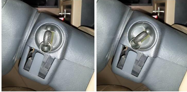
Figure 74: The ignition switch in the off position (left), and in the on position (right).
