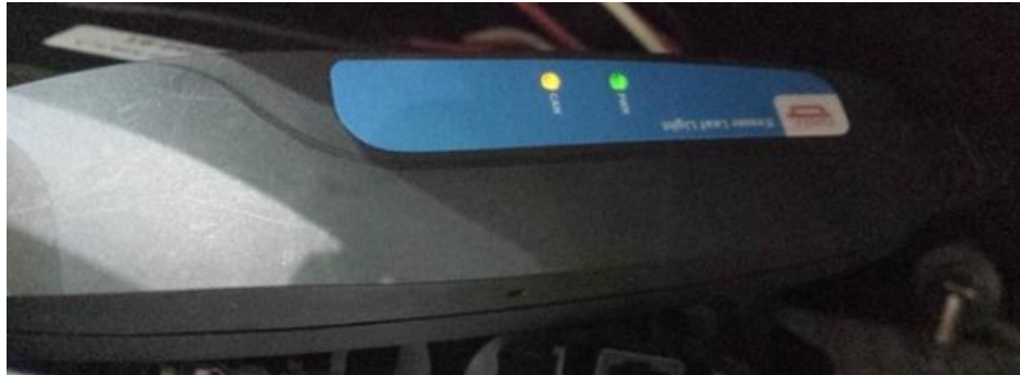
Figure 81: The green LED indicates that the adapter is powered; while the amber LED indicates the CAN bus connection has been established.
