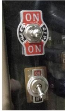
Figure 99: The regenerative braking toggle switch is located below the toggle switch for the vehicle's lights.
