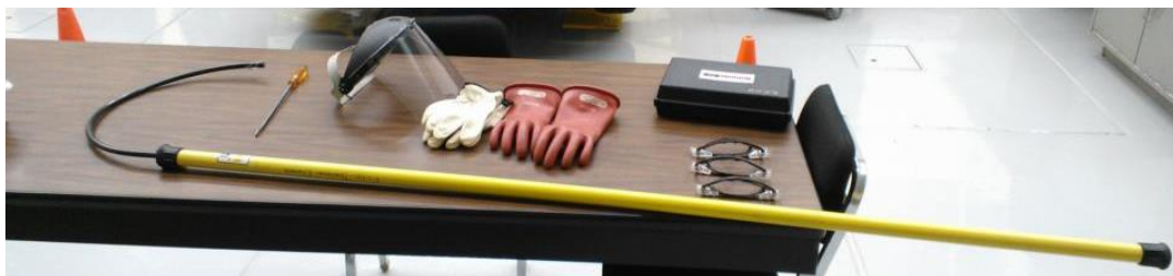
Figure 42: Electrical hook, isolating gloves, facemask, and other proper safety tools for working on Hybrid and Electric Vehicles.
