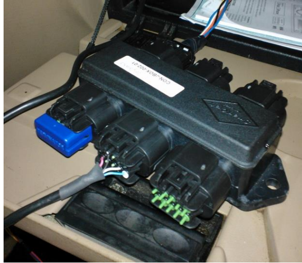
Figure 39: The Smartcraft connector has six terminals that display the same data on each pin.
