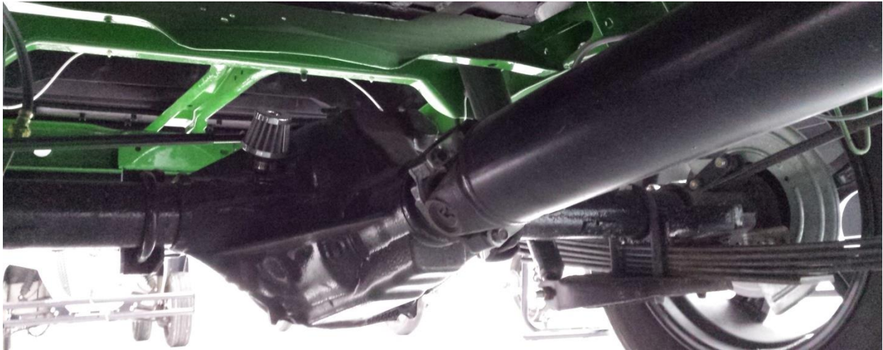
Figure 51: The JimmE-V rear differential. The motor directly drives the wheels through the rear differential. This allows the rear wheels to rotate at different speeds while turning.
