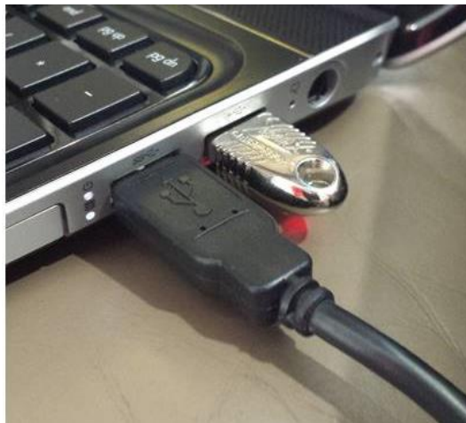
Figure 80: The Kvaser CAN adapter is connected to the laptop using the USB port next to the Crypto-Box USB drive.
