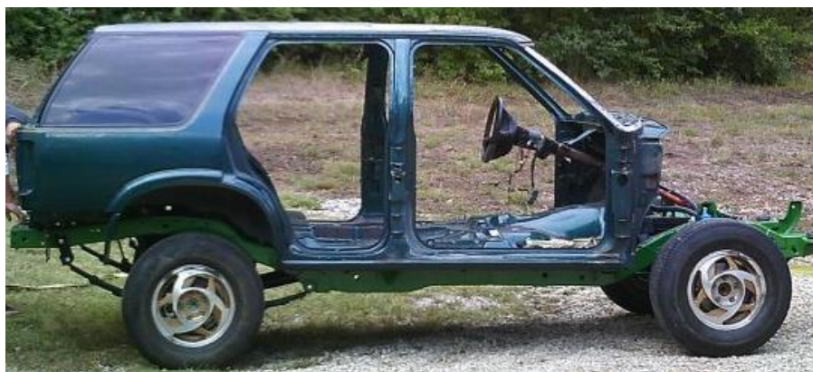
Figure 176: The original body shell installed on the recycled frame.
