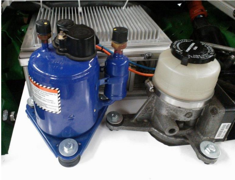
Figure 159: The electric power steering pump was installed on a steel plate in the front of the vehicle to locate the pump close to the steering gearbox.
