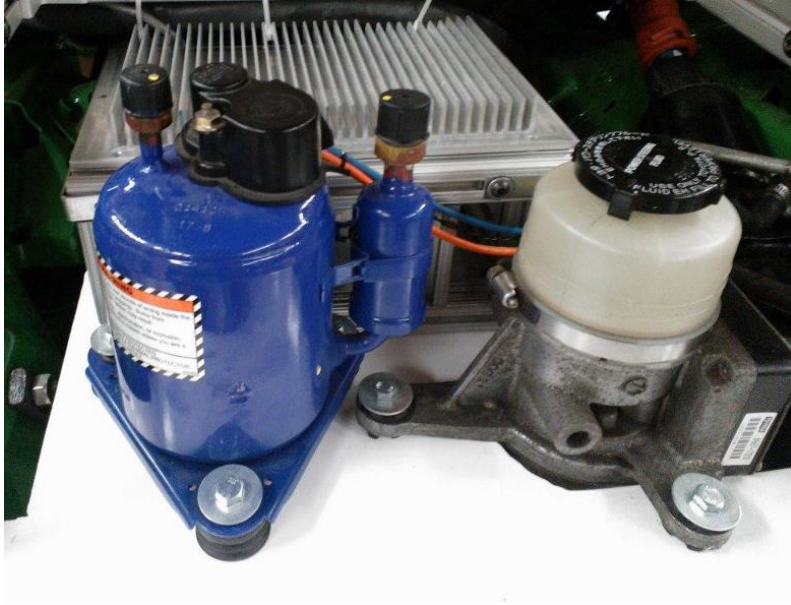
Figure 164: The electric AC compressor (left) and electric power steering pump (right).
