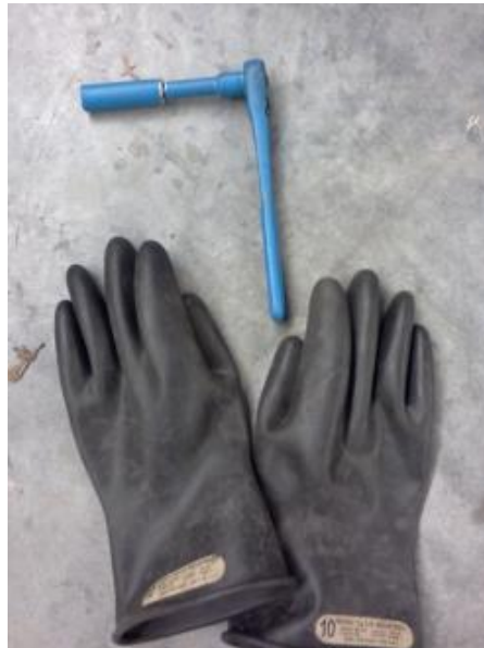
Figure 108: HV isolating gloves, and the rubber dipped tool for working on the JimmE-V battery pack.
