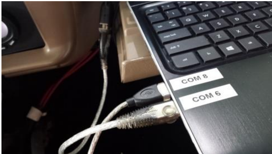
Figure 62: Connect the DMOC USB cord to COM 6 on the vehicle's laptop. COM 8 is used for the Elithion BMS.
