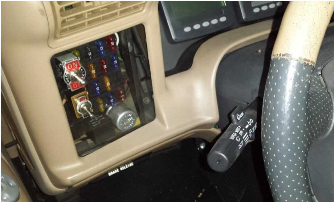
Figure 147: The main 12 VDC fuse block is installed in the dashboard to the left of the steering column.
