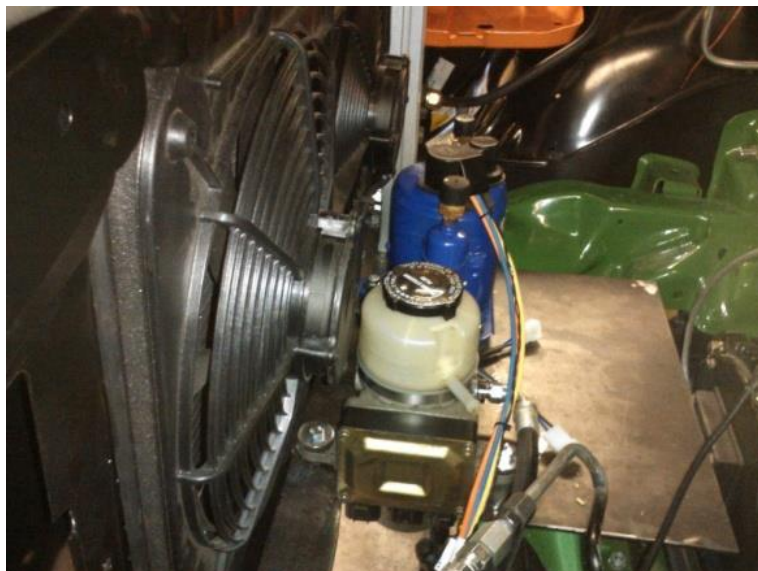
Figure 168: The AC condenser and fans are installed in the front of the JimmE-V. They are located behind the front grille to provide sufficient airflow.
