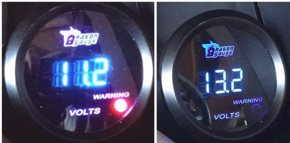
Figure 156: The 12 VDC gauge indicating a low battery (left) and a charging battery (right).
