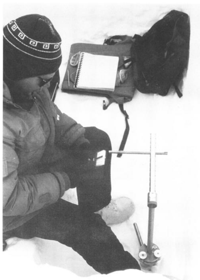
Figure 5. Collecting snow samples in cuvette tubes from a snow pit wall using an apparatus which ensures exact vertical alignment from a bubble level on the base.
