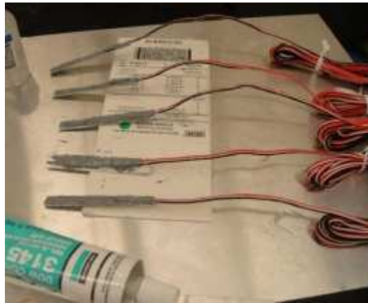
Fig. 5.3.5 Pavement strain gages (PVST)
