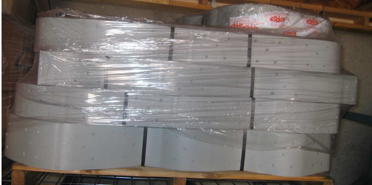
(a) Bundled geocell during transportation
