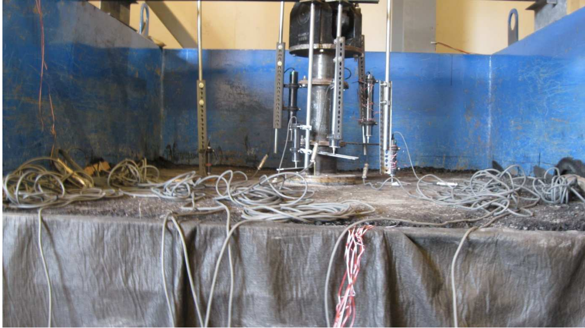
Fig. 5.3.6 Test setup for paved road test sections
