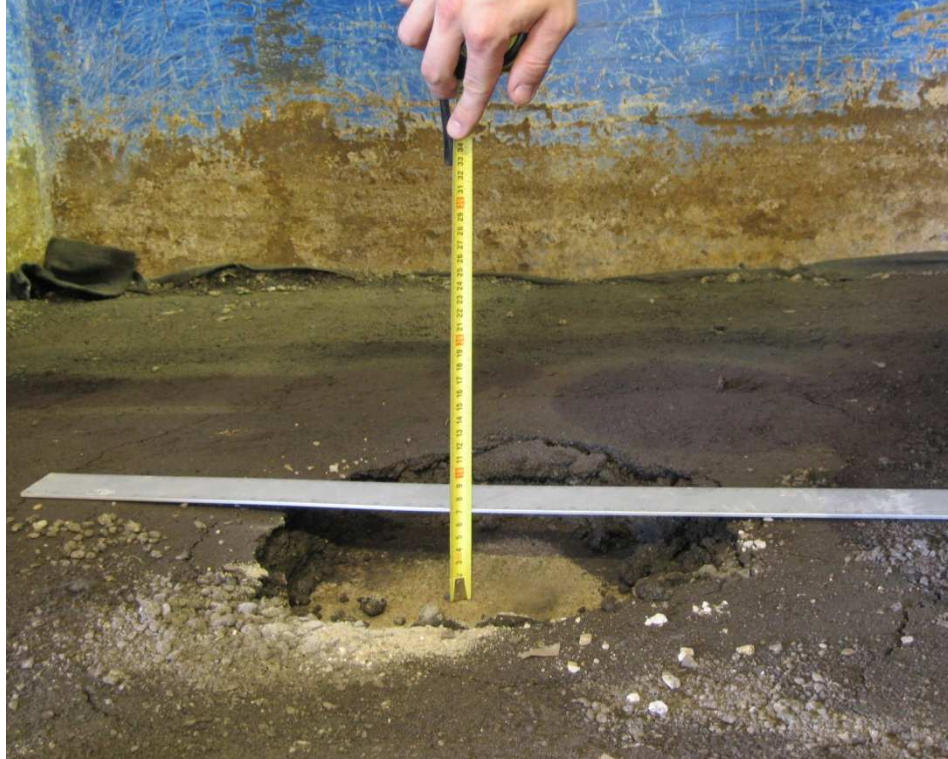
Figure 4.3.12 Displacement measurement after the cyclic plate loading test
