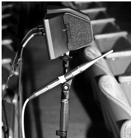
Figure 1. Binaural and omnidirectional microphones. PZM binaural assembly (top) and Earthworks omnidirectional (bottom).
