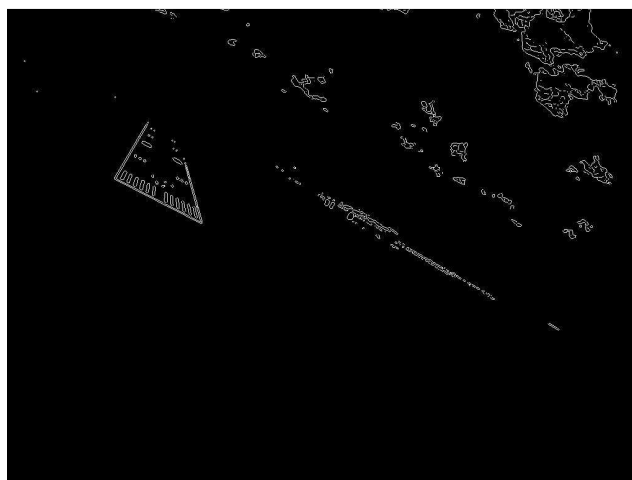
Figure 2.8: Results of Canny Edge Detector with \sigma = 1 and t = 10\% on a Sample Image
