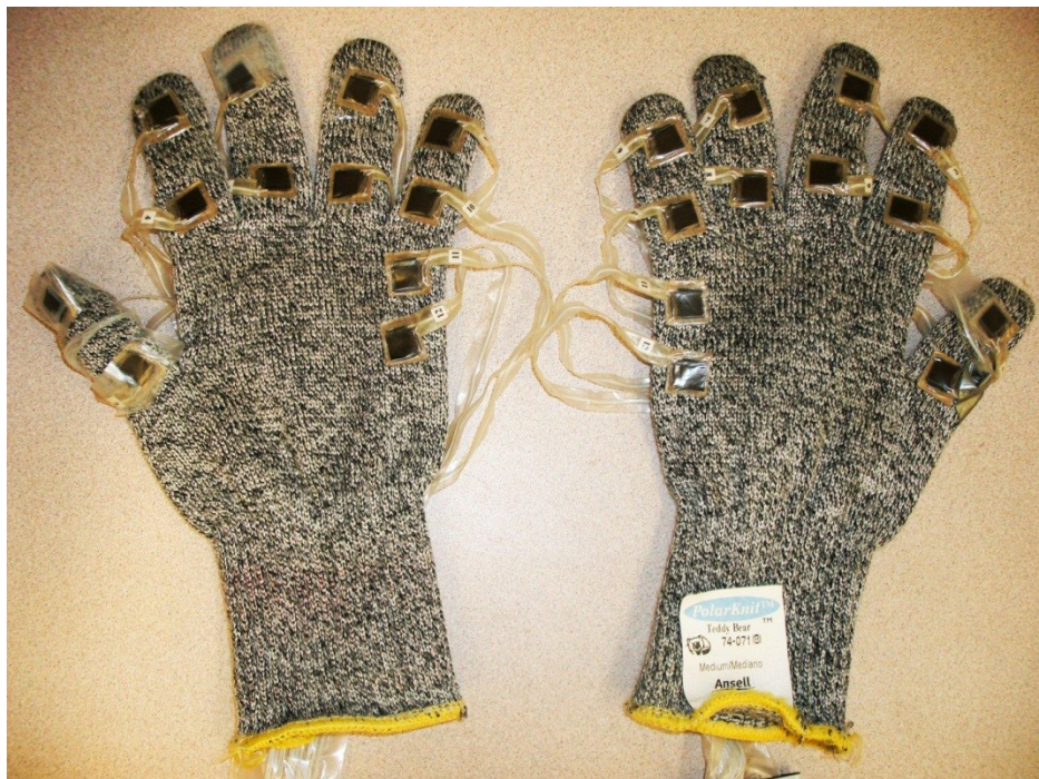
Figure 10: Photograph of the FSA glove system showing the sensors fastened on each hand. The sensors are square in shape (8mm x 8mm) and covered by Teflon.
