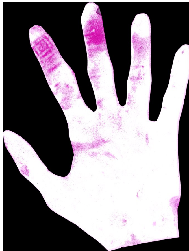
Figure 12: Illustrative example of the color density map that appeared once the film developed. In this example, the largest pressures are recorded near the tips of the fingers (darkest red).
