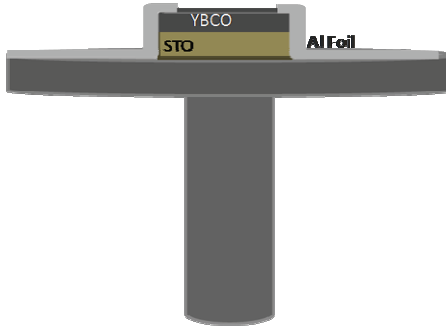
Figure 2.7: Side view of sample mounted for TEM foil preparation by FIB [52].
