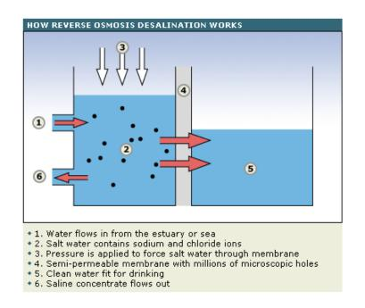
Figure 2 How Reverse Osmosis Desalination Works (Leyne, 2004). This diagram shows the basic process of the reverse osmosis desalination which the Ashkelon plant uses.
