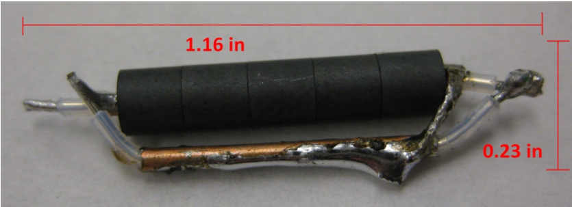
Figure 34: 1:4 Equal Delay Unun Transformer Implementation – Straight
