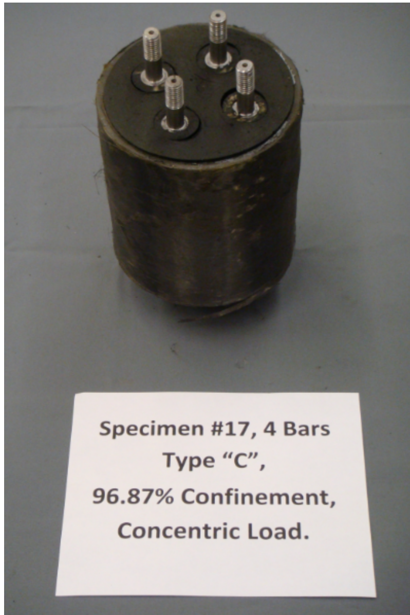
Fig. I11 - 4-Bar Type C, 96.87% Confinement Ratio, Concentric Load, Specimen #17.
