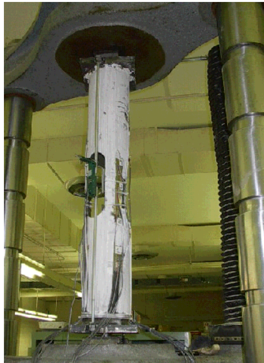
Fig. B6 - Monotonic Tension, Test Set Up.
