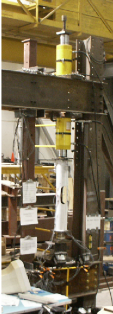
Fig. B12 - Cyclic load, Test Set Up.
