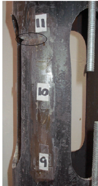
Fig. B8 - Monotonic Tension, RXS after Fracture Failure.
