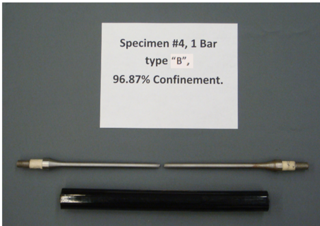
Fig. I4 - 1-Bar Type B, 96.87% Confinement Ratio, Specimen #4.
