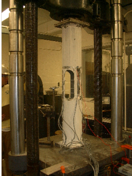
Fig. B3 - Monotonic Compression, Test Set Up.
