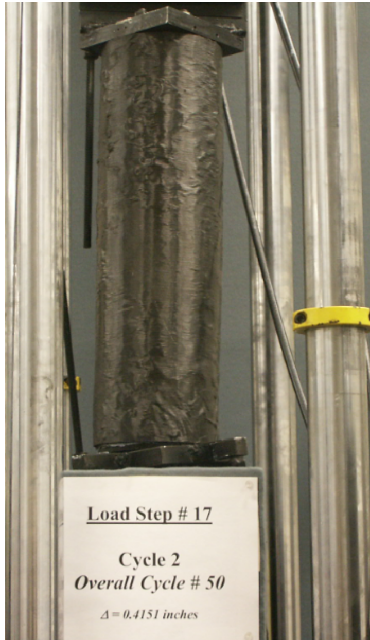
Fig. H6 - 4-Bar Fuse, Bar Type A, Confinement Ratio 98.96%, Specimen #11, Compression Cycle #50, Concentric Load.
