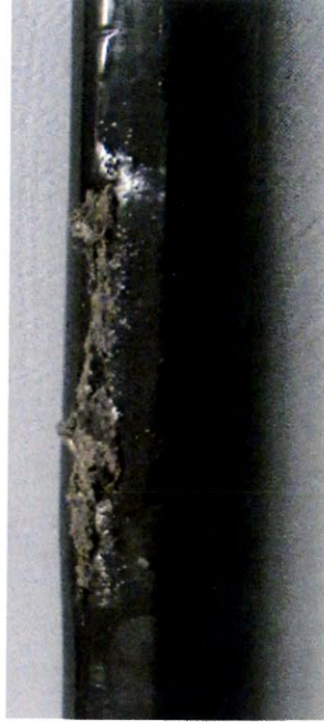
Fig. I6 - 1-Bar Type A, 98.70% Confinement Ratio, Specimen #1.
