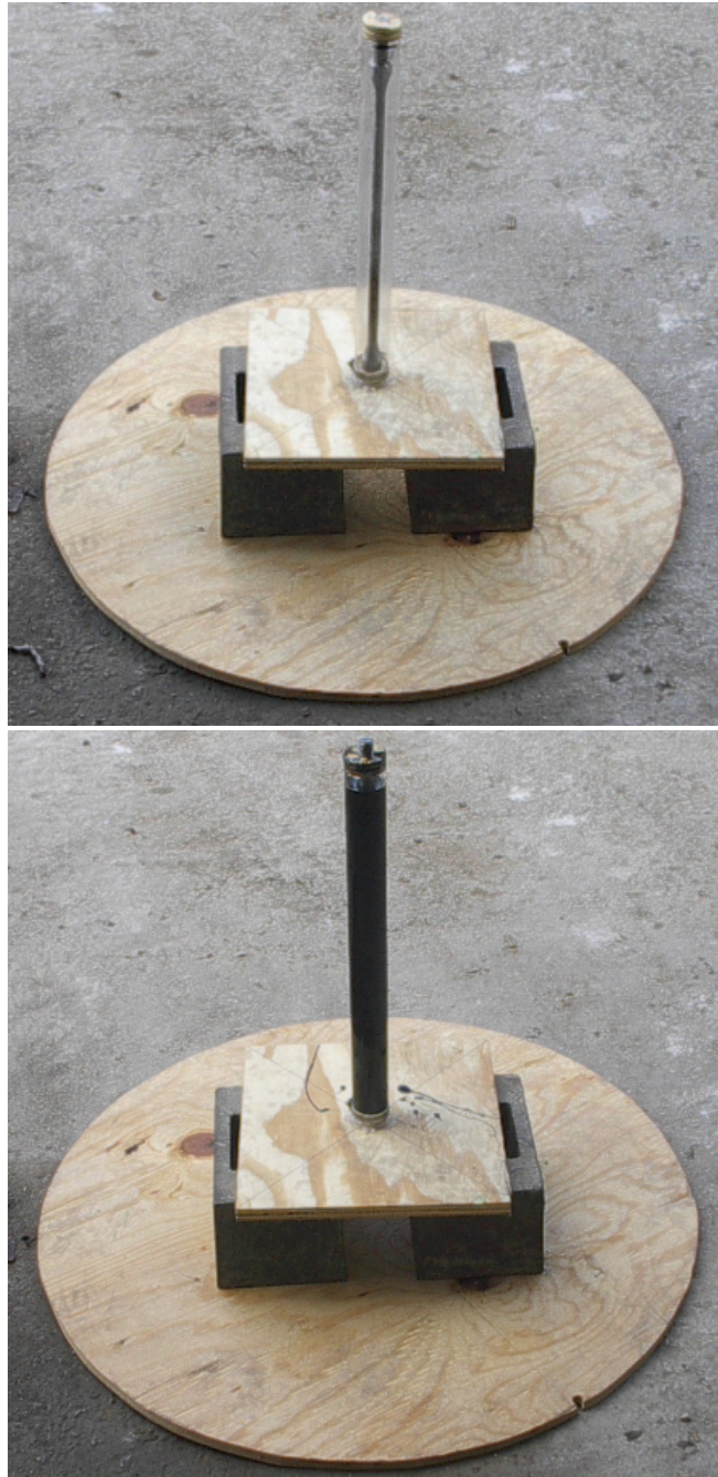
Fig. E4 - Inner Core, Bar Type B, Fabrication, before and after Pouring Castable Urethane.
