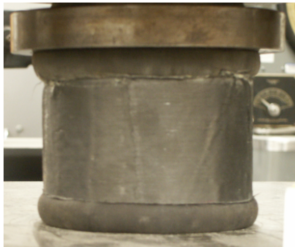
Fig. J2 - FRP-Matrix Confinement System, 60% Confinement Ratio, Monotonic Compression Test at 0.1 in./in.
