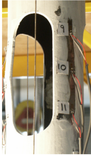
Fig. B13 - Cyclic loading, Initial Buckling Deformation.
