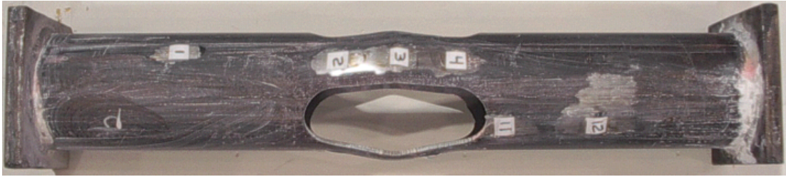
Fig. 5.9a - Monotonic Compression, RXS after Buckling Failure.
