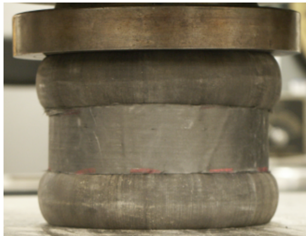
Fig. J3 - FRP-Matrix Confinement System, 30% Confinement Ratio, Monotonic Compression Test.
