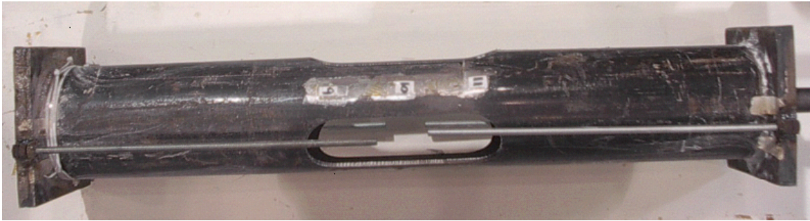
Fig. B7 - Monotonic Tension, Test Specimen after Fracture Failure.
