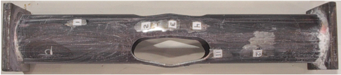
Fig. B4 - Monotonic Compression, Test Specimen after Failure.
