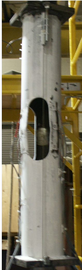
Peak deformation under tension last cycle load step #9
