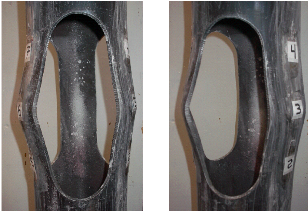
Fig. 5.9b - Monotonic Compression, RXS after Buckling Failure.
