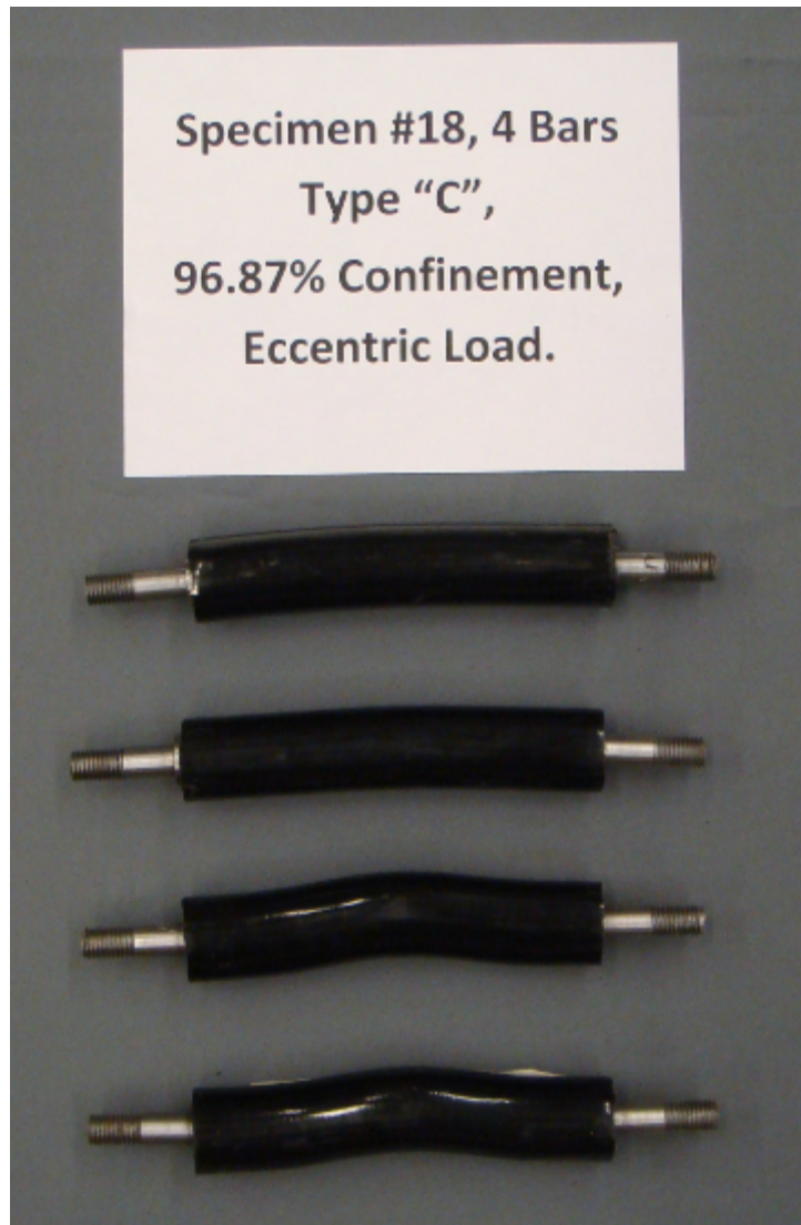
Fig. I7 - 4-Bar Type C, 96.87% Confinement Ratio, Eccentric Load, Specimen #18.
