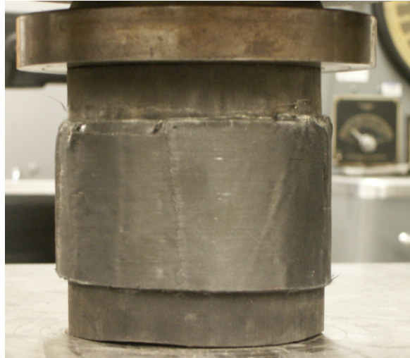
Fig. J1 - FRP-Matrix Confinement System, 60% Confinement Ratio, Monotonic Compression Test.
