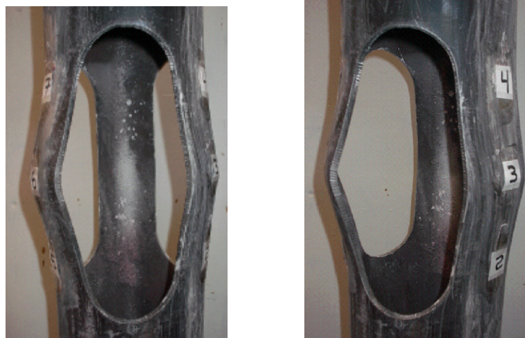
Fig. B5 - Monotonic Compression, RXS After Buckling Failure.
