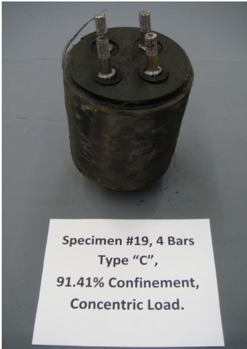
Fig. I10 - 4-Bar Type C, 91.41% Confinement Ratio, Concentric Load, Specimen #19.
