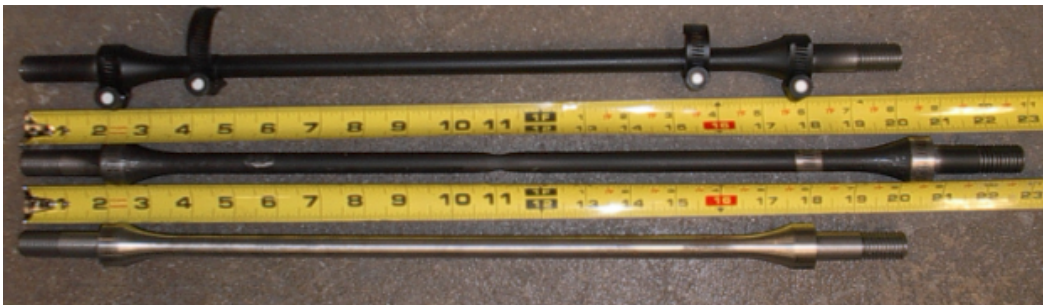
Fig. 8.4 - Monotonic Tension Test Specimen Inelastic Deformation.
