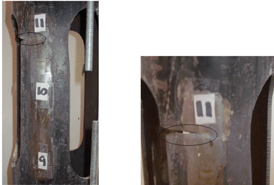
Fig. 5.17 - Monotonic Tension, RXS after Fracture Failure.
