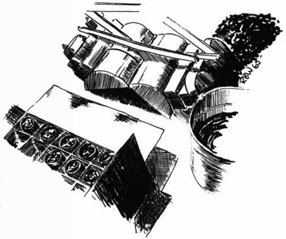
FIG. 4. Sampling equipment, including 200 ml. sample bottles in box and Peterson dredge in open position.
