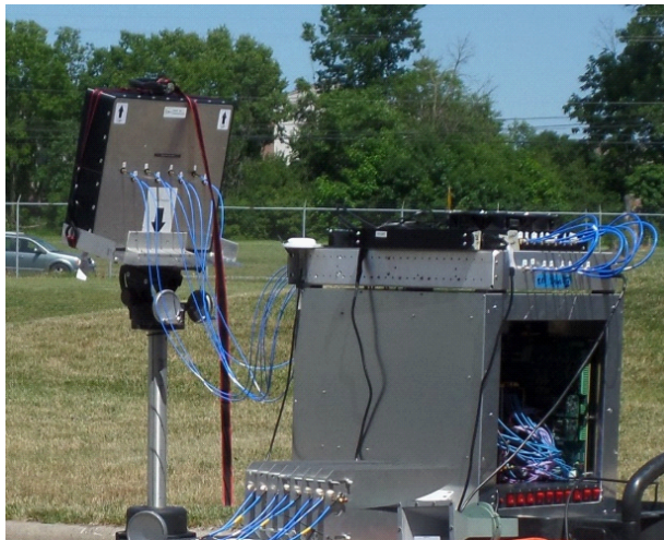
Transmitter front end and antenna
