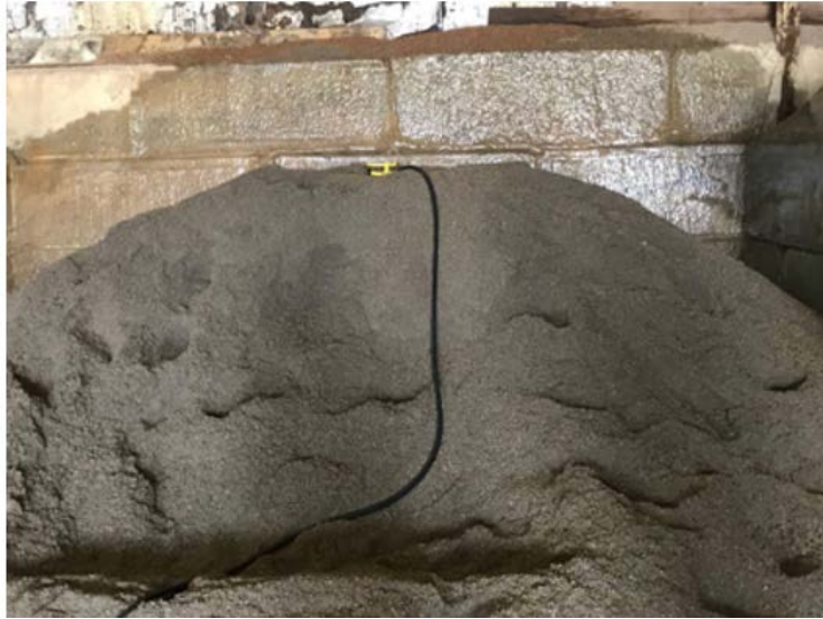
Figure 2.8: Lightweight Aggregate Stockpile for MN-IC-LC-HPC-5
