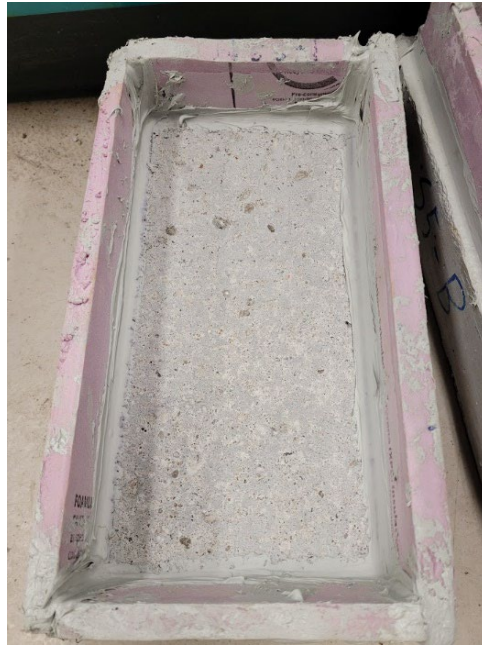
Figure 2.2: Scaling resistance test specimen with foam dikes attached
