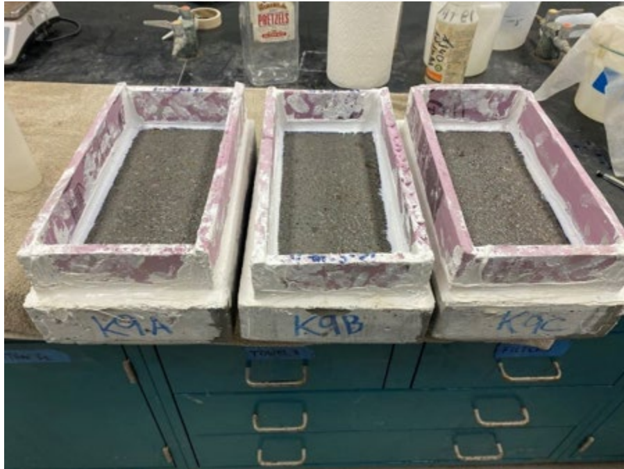
Figure 2.5: Scaling specimens with polystyrene foam dikes attached
