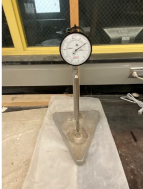
Figure 2.2: Mechanical dial gauge length comparator
