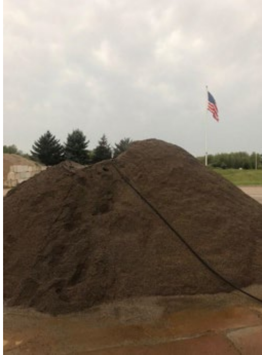
Figure 4.15: Lightweight aggregate stockpile for MN-IC-LC-HPC-6
