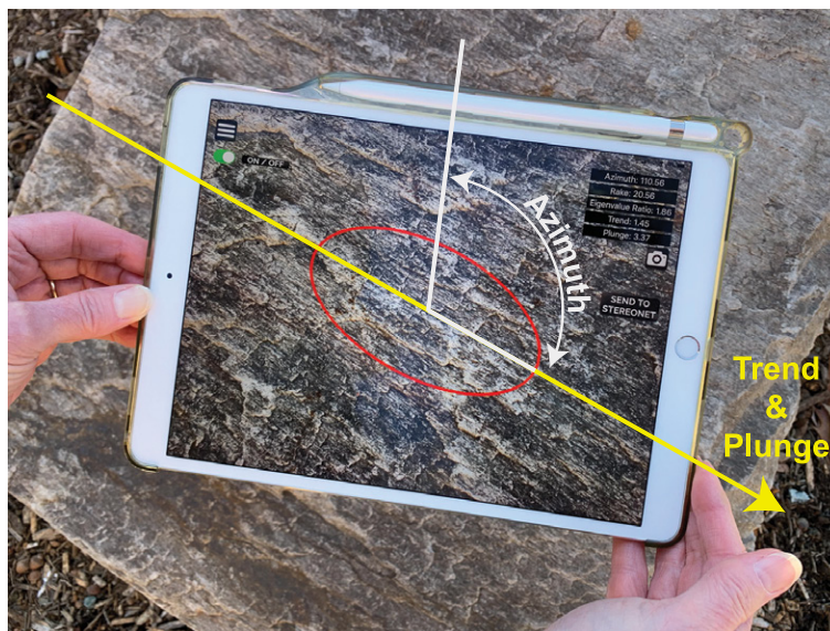
Figure 3. Using the edge fabric tool. The mobile device is held parallel to the plane being photographed. The app calculates the edge fabric ellipse and reports its azimuth (long axis of the ellipse, relative to “up” on the screen), its trend and plunge in space, and its axial ratio E . Calculations take 5 seconds or less. The analysis can be captured as a screenshot, and the trend and plunge can be copied for pasting into Stereonet Mobile (Allmendinger, 2019). StraboTools locks to landscape display.
