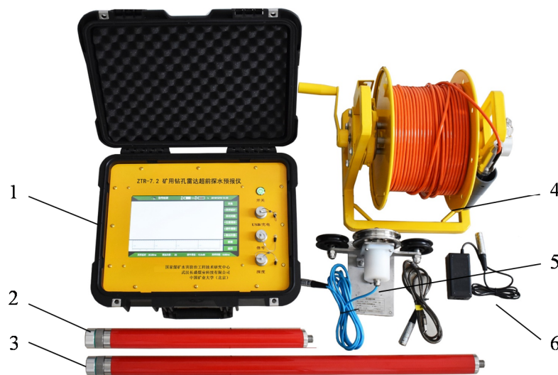
Figure 2. The single borehole ground penetration radar (GPR) prototype system. 1—computer, 2—transmitting antenna, 3—receiving antenna, 4—fiber cable, 5—depth counter, 6—charger.
