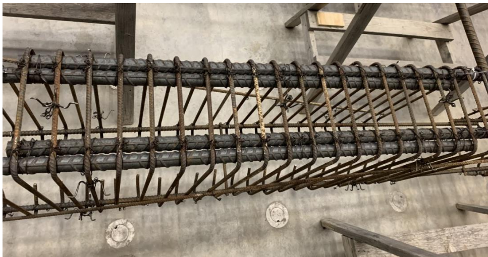
Figure 3.5: Heavily confined lap splice (14-g)
