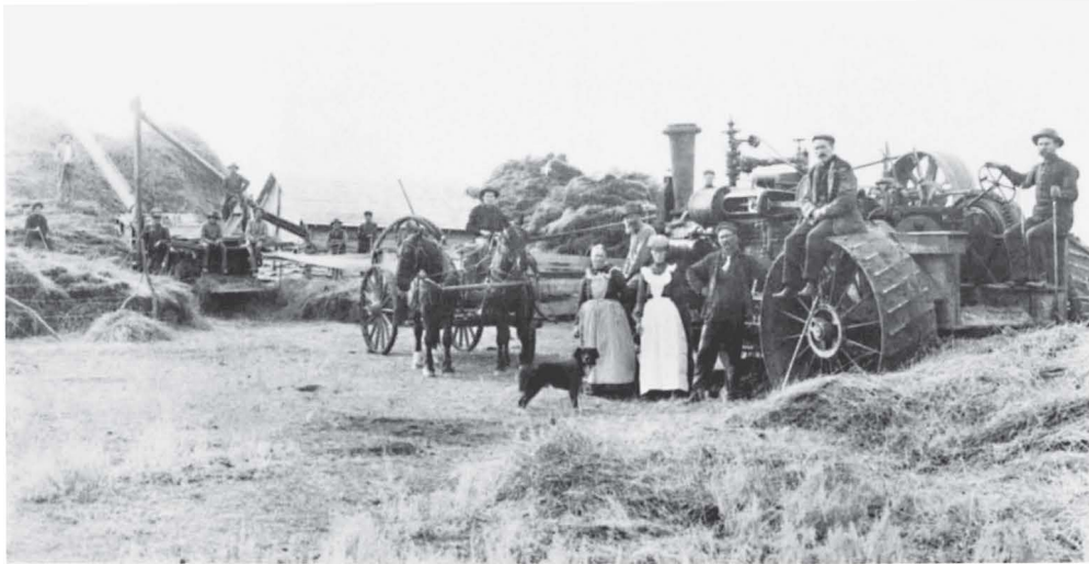
The Holden brothers outfit of Indian Head, Sask., had no self-feeder in 1903, and so a band cutter and feeders fed the thresher. The engine was a straw burner; hence the pile of straw behind the engineer. (Provincial Archives of Saskatchewan)
