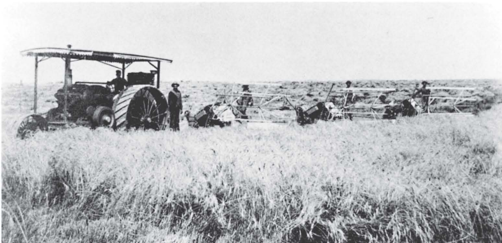
Three binders and five men with an oil-pull tractor on the William Phillips farm, Belpre, Kans., ca. 1920. (Santa Fe Trail Center, Larned, Kans.)
