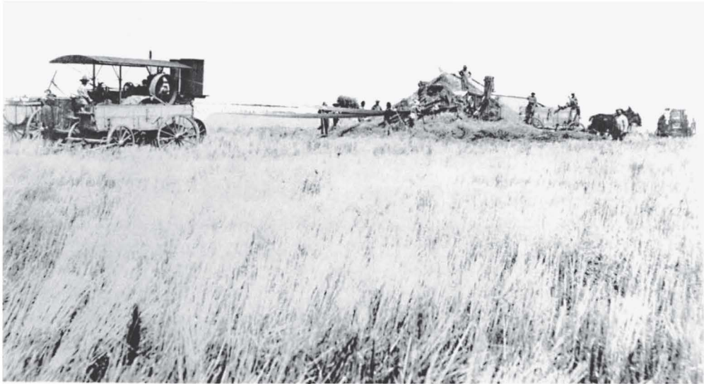
The long belt sets the engine at a distance from the stacks. An outfit near Belpre, Kans., ca. 1910. (Santa Fe Trail Center, Larned, Kans.)
