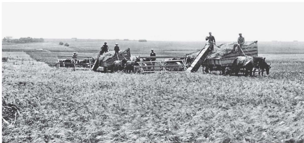
Heading wheat on the John Thielen farm, central Kansas, July 9, 1909. The header was the machine for big farms in the winter wheat region. (Halbe Collection, Kansas State Historical Society, Topeka)
