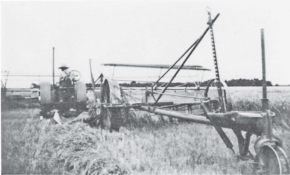
Header, with the elevator removed, being used as a swather in Thomas County, Kans., 1929. (Courtesy of Franz Goossen)
