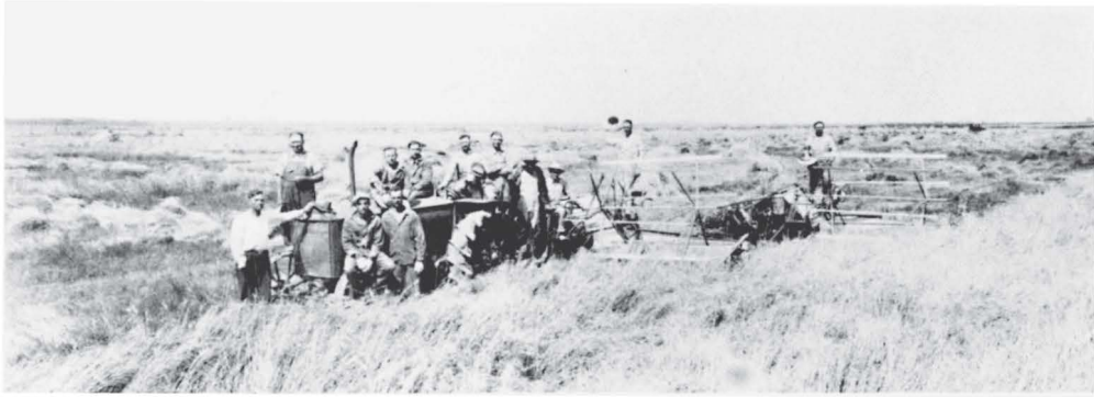
Binders hitched in tandem by G. L. Mumma near Dighton, Kans., ca. 1925. (Lane County Historical Museum, Dighton, Kans.)
