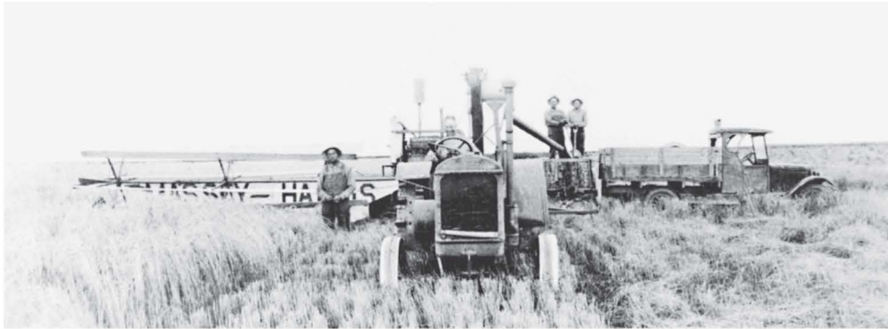
Prairie combine with auxiliary engine in Lane County, Kans., 1928. (Lane County Historical Museum, Dighton, Kans.)
