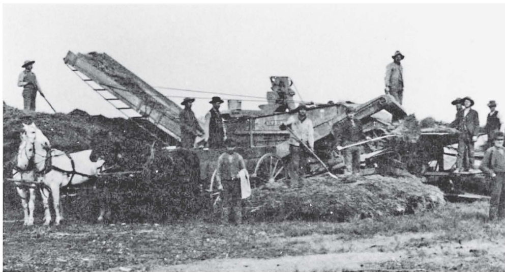
Two feeders and a band cutter are in place here to feed the bundled grain from the stack. Shown is the C. R. Voth outfit, Harvey County, Kans., ca. 1900. (Courtesy of Moses Voth)
