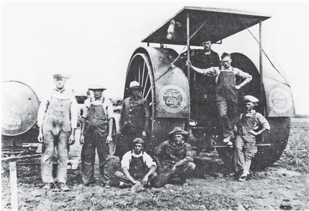
A fuel tank replaced the coal car on the Voth outfit, ca. 1910. (Courtesy of Moses Voth)
