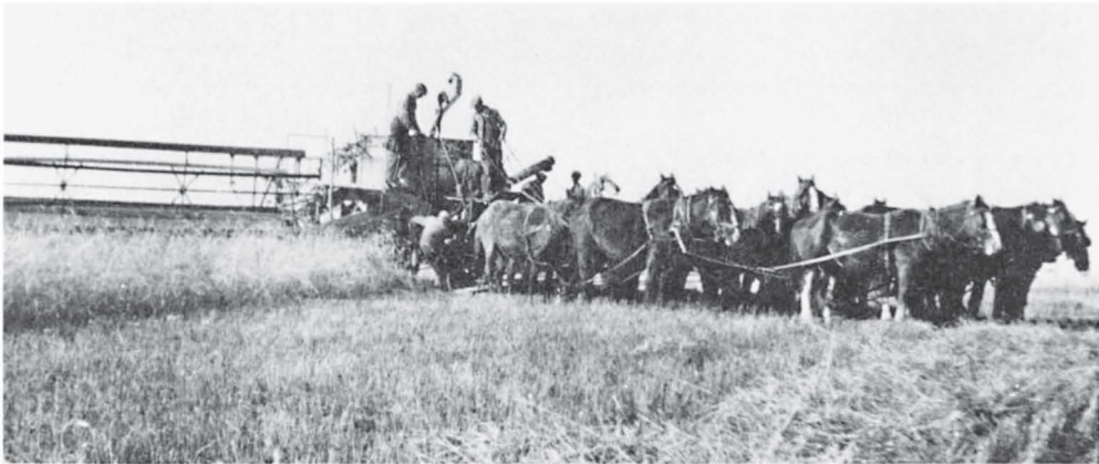
Twenty-foot, horse-drawn, ground-wheel-driven Holt combine at Ensleigh, Alta., 1927. (Glenbow Archives)
