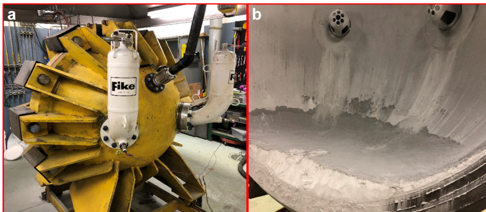
Figure 12. Test setup for a 1 m 3 suppression testing with two 10 L HRDs (a) and residual combustion deposit following active suppression of aluminum deflagration with Met-L-X suppressant agent; Test Series 5 (b).
