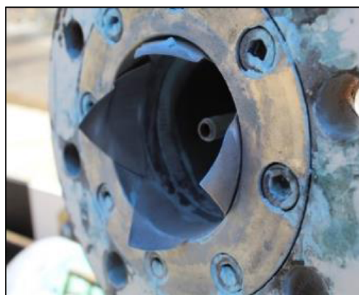
Figure 10. Post-test evaluation; validation that HRD rupture disc opening is complete and nonfragmenting; Test No. 1-R1 with SBC.
