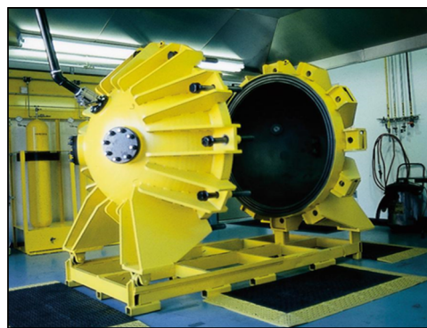
Figure 5. Fike Corporation 1 m 3 combustion test vessel, utilized for fuel explosibility and active suppression testing.
