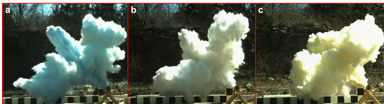
Figure 7. Comparison of plume geometries during open-air discharge testing, including Test No. 1-R1 with SBC (a), Test No. 2 with Met-L-X (b), and Test No. 3 with MAP (c); images captured at 75 ms following system activation.
