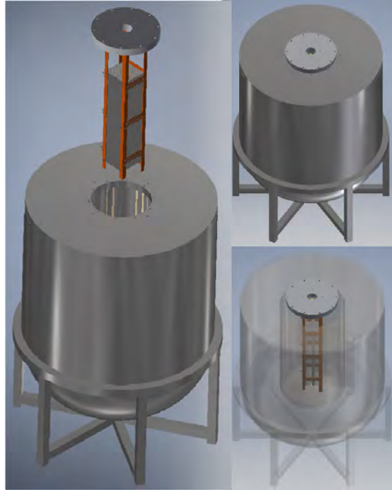
Figure 7: Images of the final design of the cryostat and field cage.
