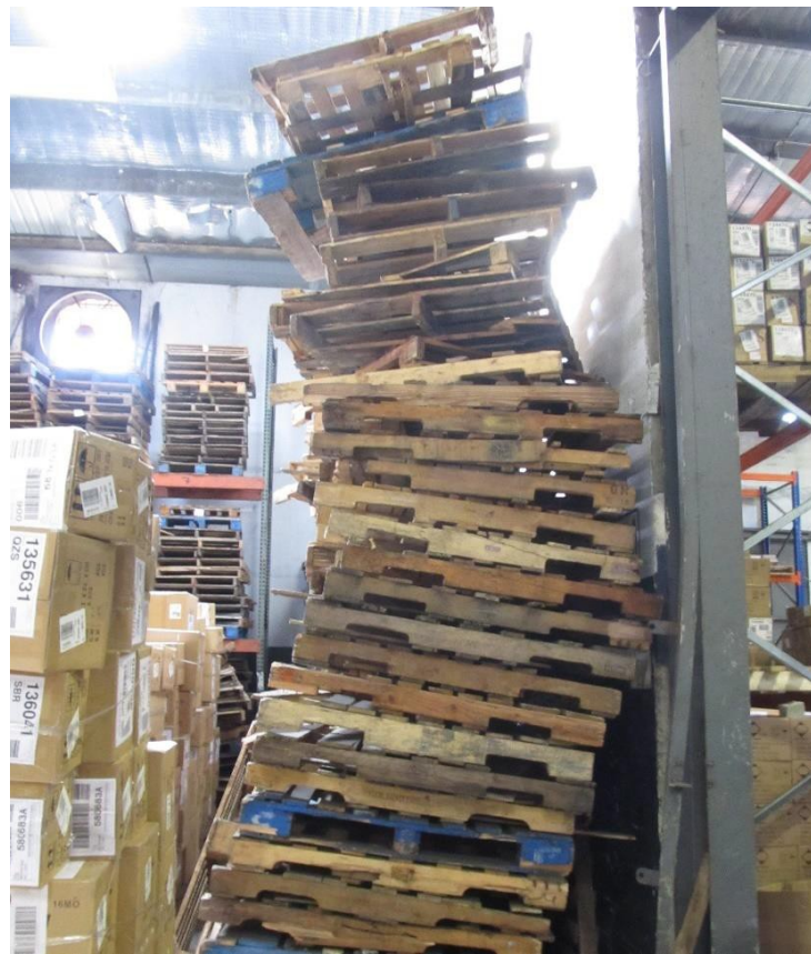
Figure 35.1: Unsafe Pallet Storage in Panama
