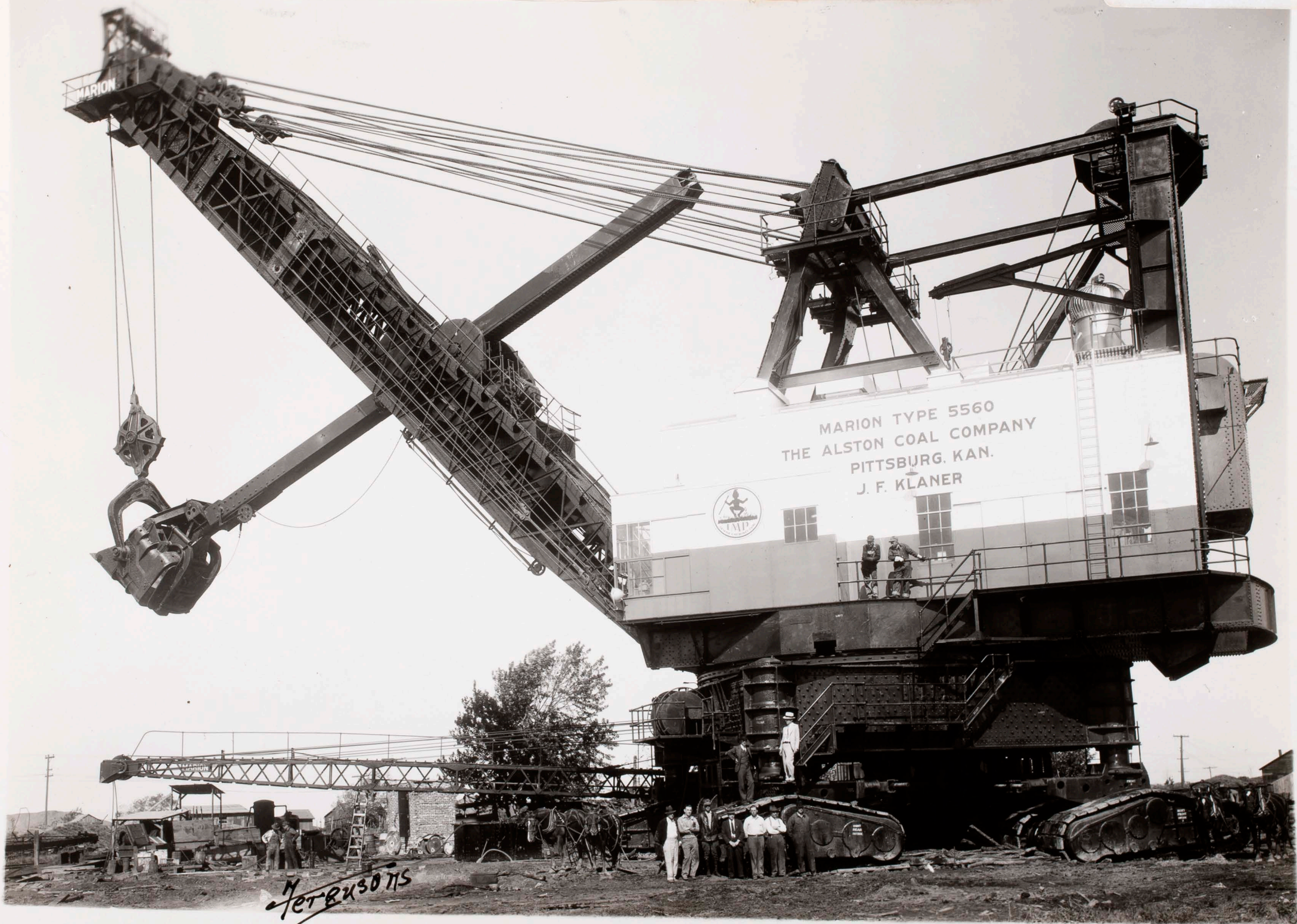
Fig. 8.--A Marion electric shovel with a 20 cubic yard dipper and a 90 foot boom. This shovel is operated near the Kansas-Missouri state line by the Alston Coal Company.
