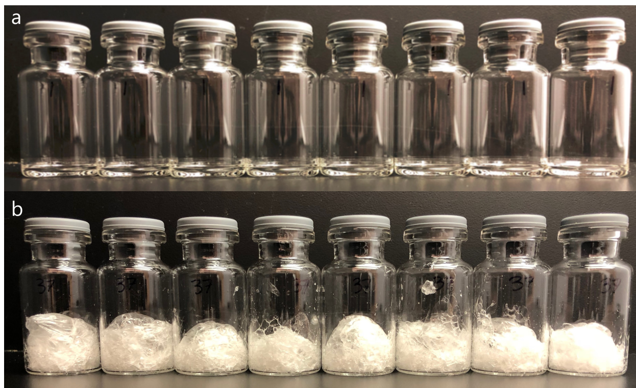
Figure 5. Comparison of product appearance for 30% sucrose solution (a) and 30% sucrose, 3% BSA solution (b) after vacuum drying cycle.
