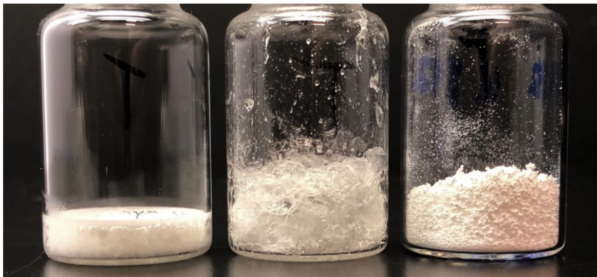
Figure 12. Freeze-dried (left), vacuum-foam dried (center) and spray freeze-dried (right) preparations of dried human T cells (Formulation: 30% trehalose, 3% BSA in PBS, pH 7.4).
