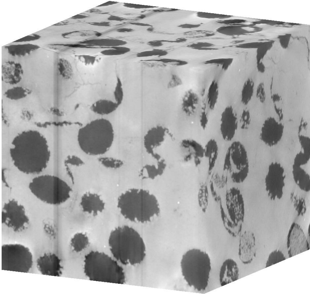
Figure 6. CT reconstruction of oomoldic grainstone sample G1. 600 image stack with a cube edge of ~ 2.6 mm.
