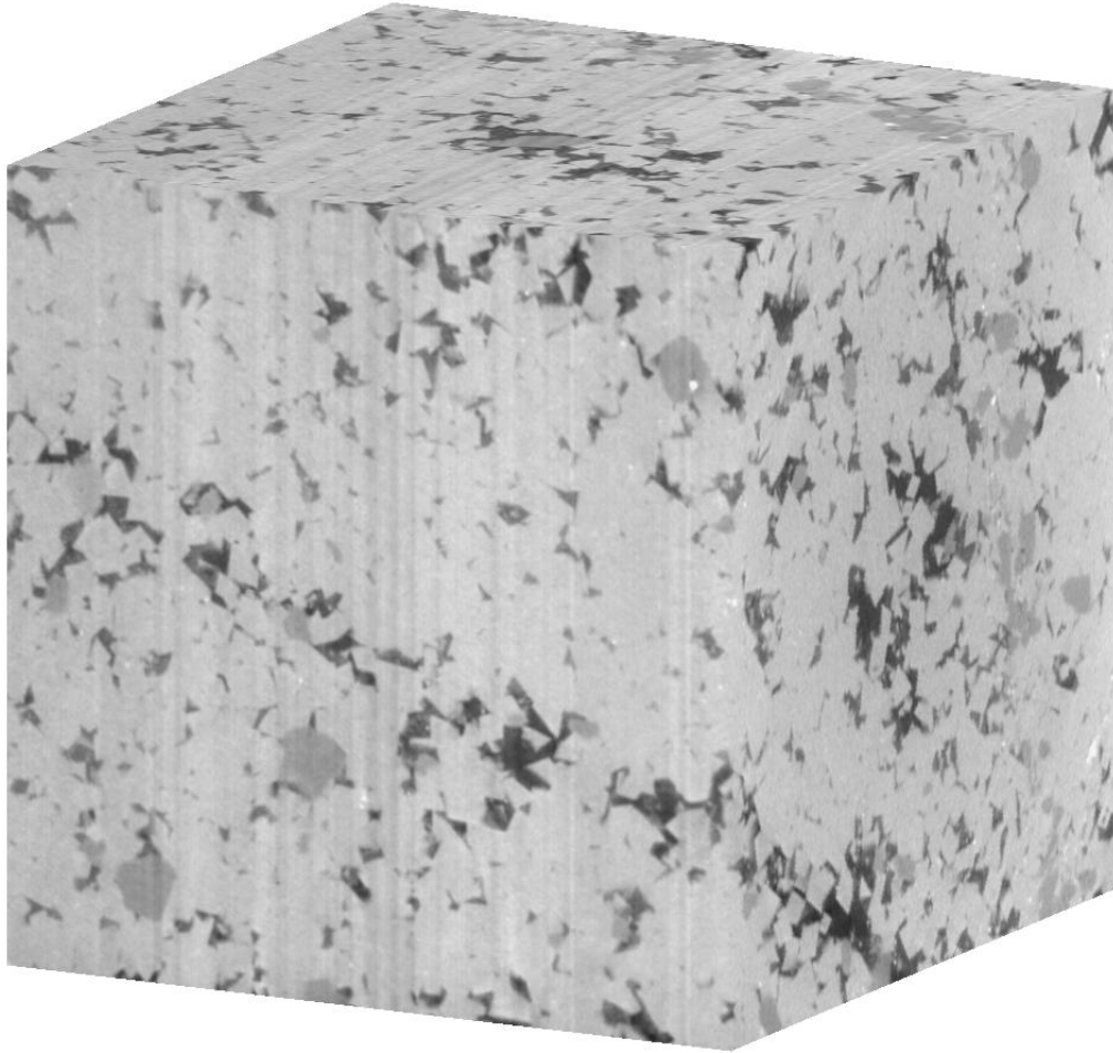
Figure 2. CT reconstruction of mudstone sample M2. 600 image stack with a cube edge of \sim 2.6 mm.
