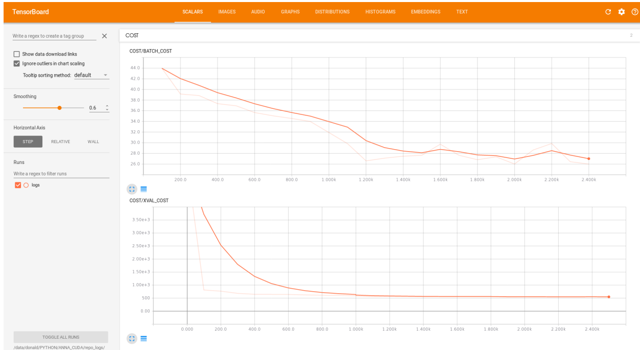
Figure 4.6: Screenshot of the cost graphs in TensorBoard. The upper plot shows the cost associated with each individual batch as a function of weight update iteration, and the bottom plot shows the same except for the cross-validation set.
