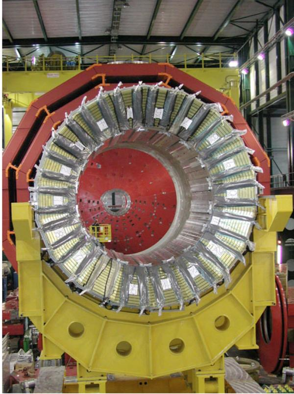
Figure 3.22: ([23], 124) Photograph of one half of HB prior to installation. The absorber layers of brass are clearly visible, as well as the gaps between them that contain the scintillator plates.
