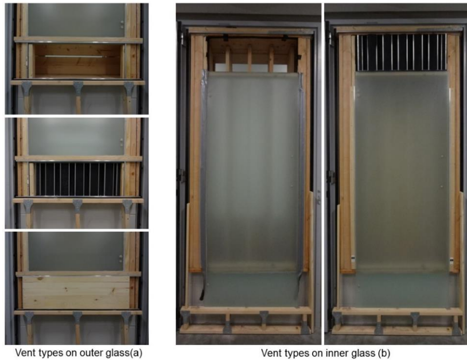
Figure 5.11 Vent types on inner glass (a) and outer glass (b)
