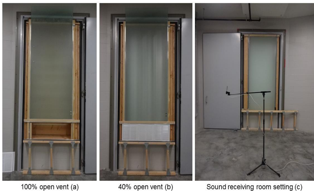
Figure 5.9 DSF mock-up setting of the sound sending (a,b) and receiving room (c)
