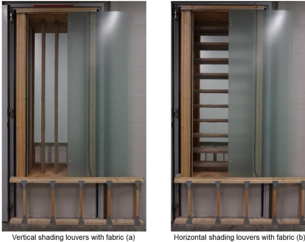
Figure 5.7 Vertical (a) and horizontal shading louvers (b) wrapped with fabric tilted at a 0 degree angle
