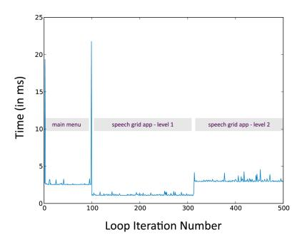
**Fig. 4.**Overall system lag for an example implementation employing the proposed framework displayed as system delay evolution over time. In this example, the BCI application entered a toplevel main menu, then entered a hierarchical speech output system with two layers. Each app (in. main menu, or speech output) utilized different levels of resources, though overall system delay averaged less than 5 ms.
