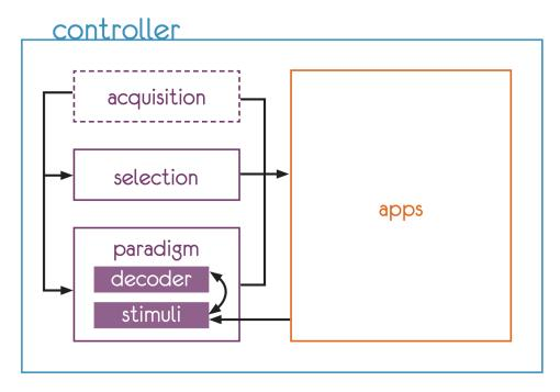
**Fig. 1.** A system diagram of the framework processing modules. Arrows indicate lines of communication between processing modules, handled in the background by a master controller. The effort here has been to isolate, as much as possible, the app environment from the remaining modules. This isolation is key for invoking a "crowd-sourcing" paradigm for BCI application development.
